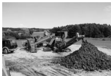
Fig. 10.2 Soil preparation unit type 'mole'.
