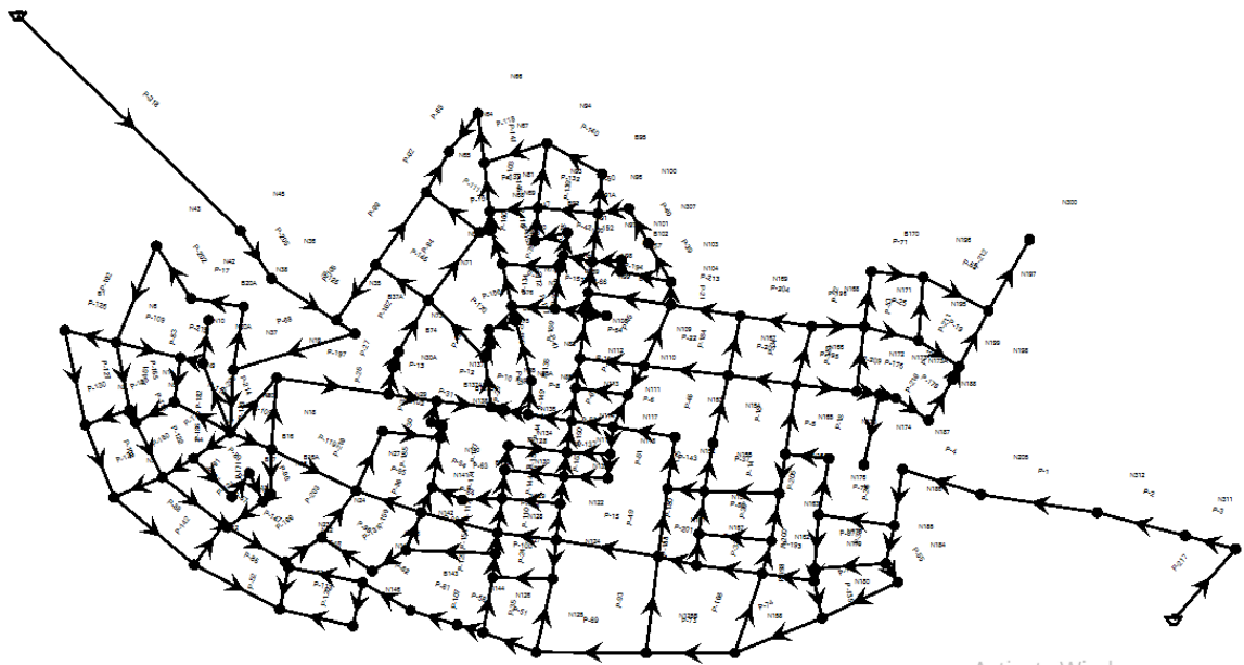
Figure 4-5: Layout of Jigjiga Town water supply system
