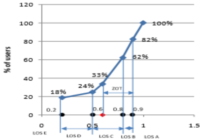
Figure 4.33: Level of service range due punctuality (source: Sherya D. and Debapratim P., 2013)
