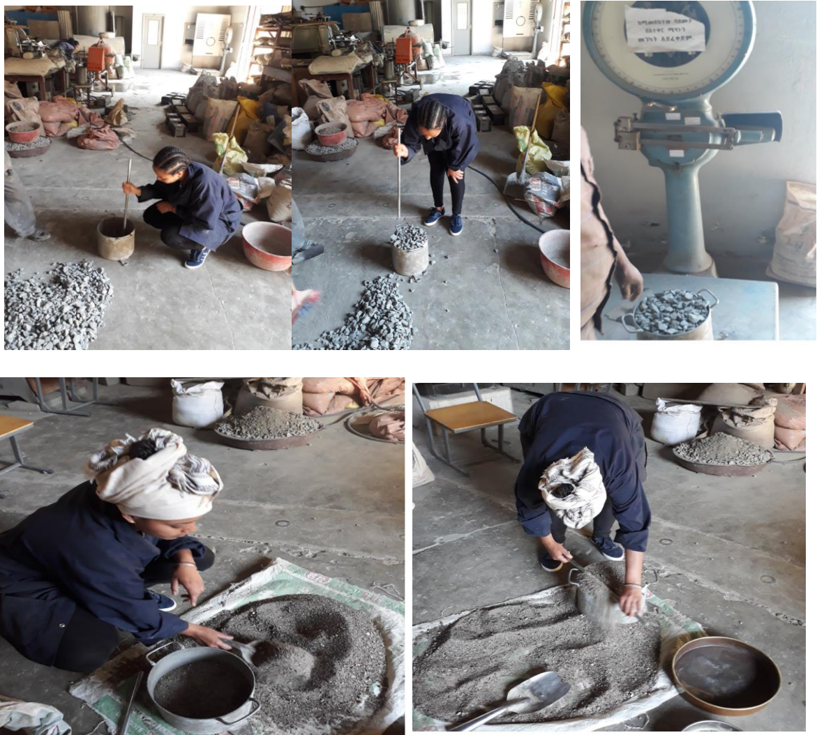
Figure 3.5. Measuring dry unit weight for both FA and CA
