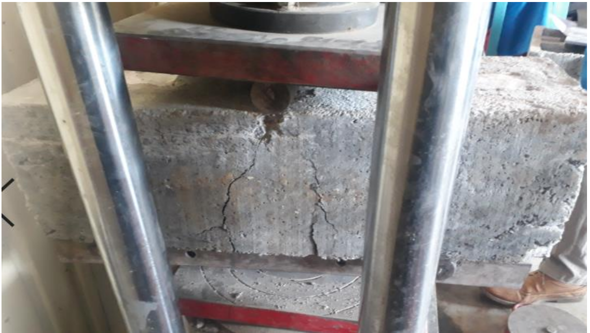
Figure C.11. Flexural strength test for RC beams
