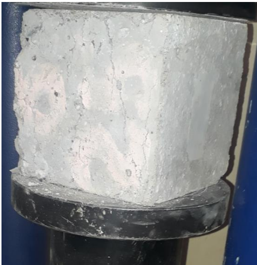
Figure 4.47. Color of specimen under 600°C and 2hr
