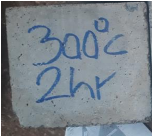
Figure 4.43. Color of specimen under 300 °C and 2hr
