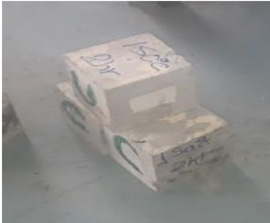
Figure 4.41. Color of specimen under 150 °C and 2hr
