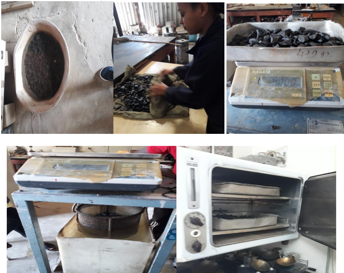
Figure 3.6. Measuring specific gravity for CA
