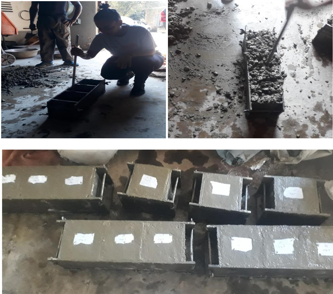
Figure 3.12. Casting of Cubes for compressive strength test
