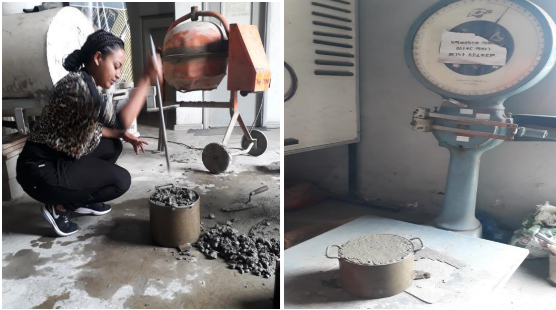
Figure 3.10. Fresh concrete unit weight Test
