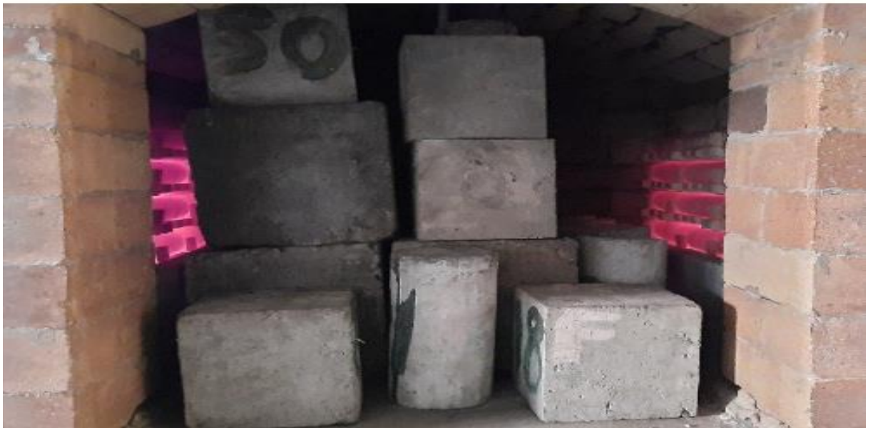
Figure C.7. Specimens inserted in furnace
