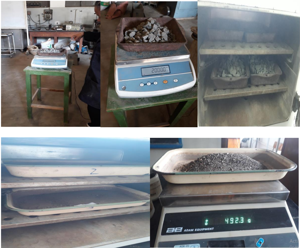
Figure 3.4. Measuring moisture content for both FA and CA
