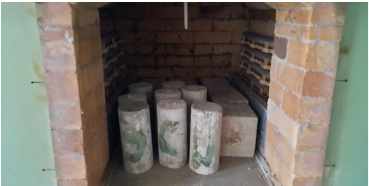
Figure 3.17. Specimen in blast furnace
