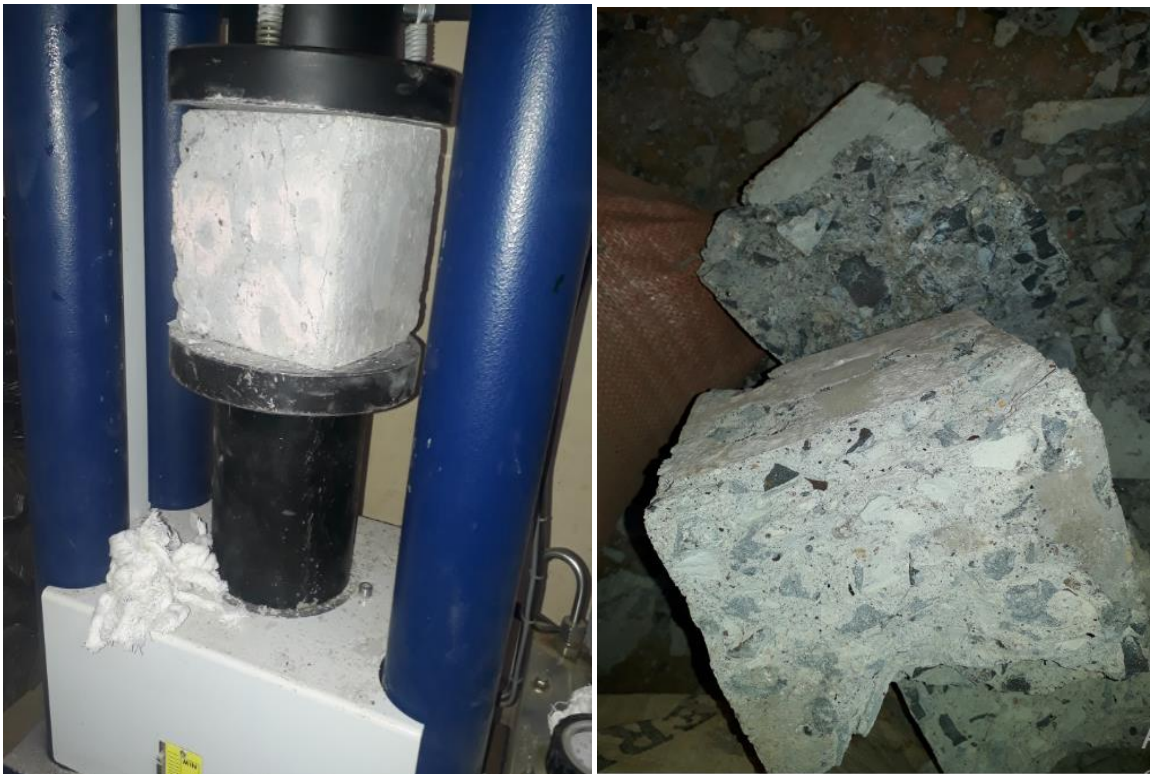
Figure C.9. Compressive strength test for cubes after exposed to fire
