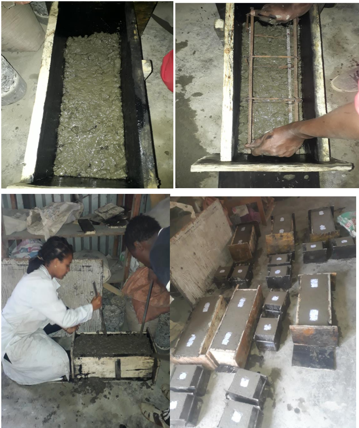
Figure 3.15. Casting of beams for flexural strength test
