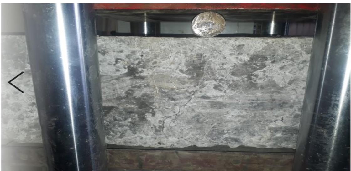
Figure 4.38. Crack of RC concrete with glass fiber
