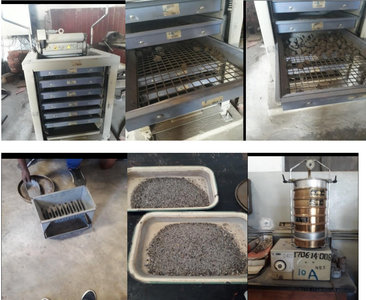
Figure 3.3. Measuring sieve analysis for CA and FA
