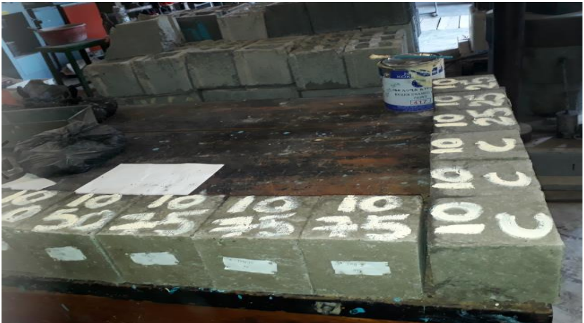
Figure C.2. Cubes casted for compressive strength test
