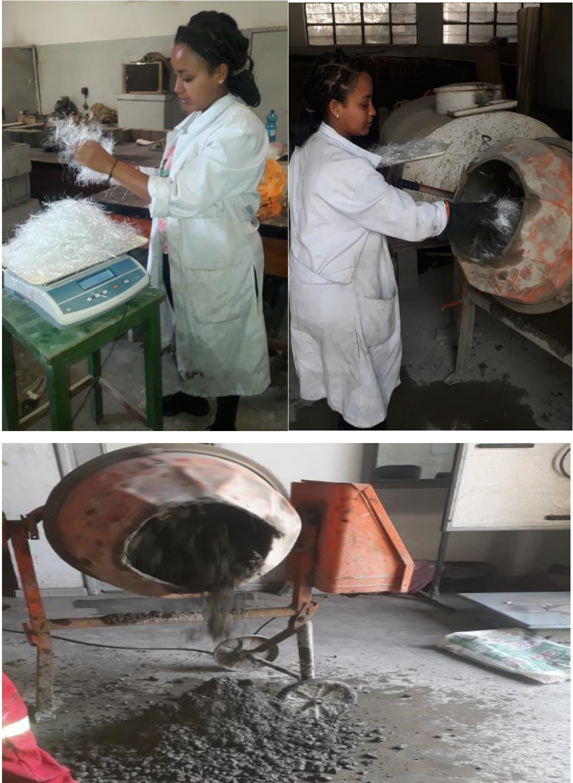
Figure C.1. Mixing of concrete with glass fiber
