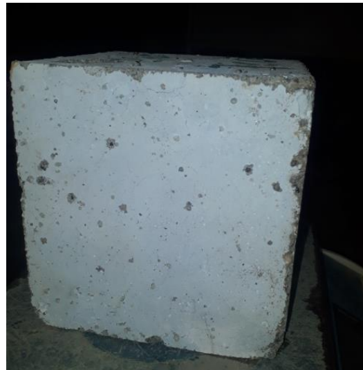
Figure 4.48. Color of specimen under 600°C and 4hr
