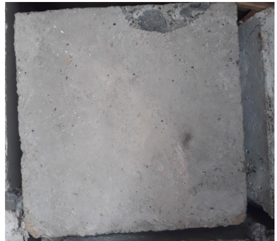
Figure 4.44. Color of specimen under 300 °C and 4hr
