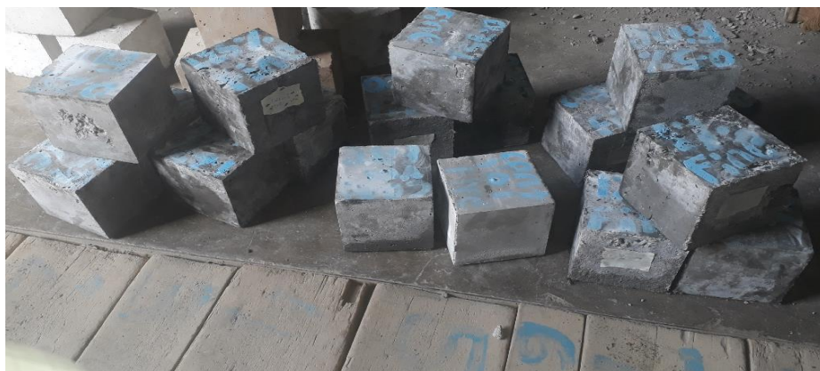
Figure 3.11. Cubes for compressive strength test
