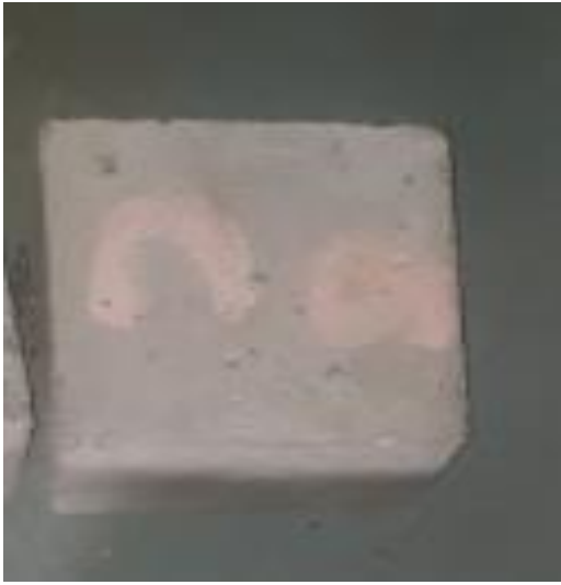
Figure 4.45. Color of specimen under 450°C and 2hr
