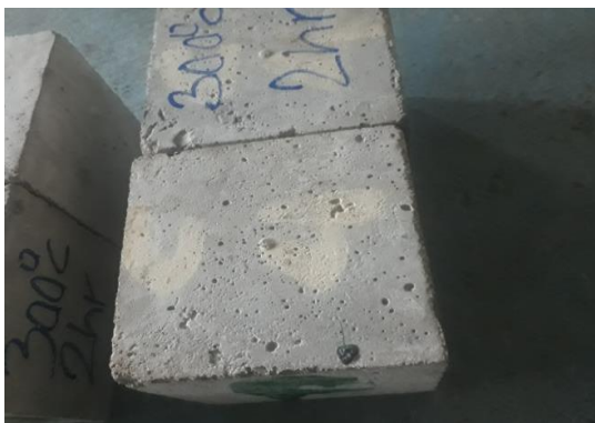
Figure 4.35. Spalling at temperature level of 300°C
