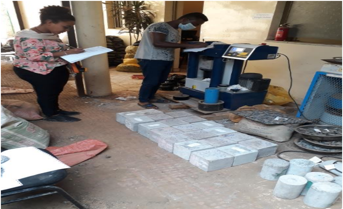
Figure C.8. Specimens after exposed to fire
