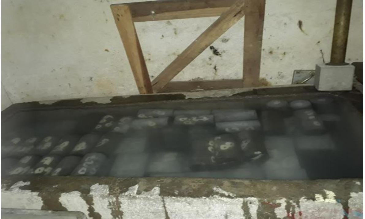
Figure C.4. Curing of specimens
