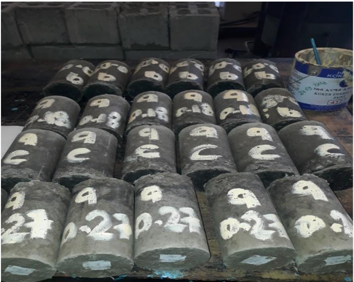
Figure C.3. Cylinders casted for split tensile strength test
