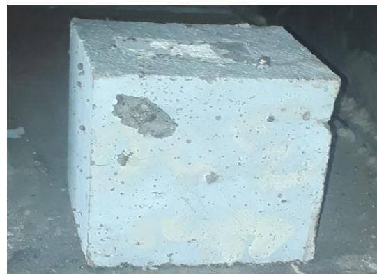
Figure 4.36. Explosive Spalling at temperature level of 600°C
