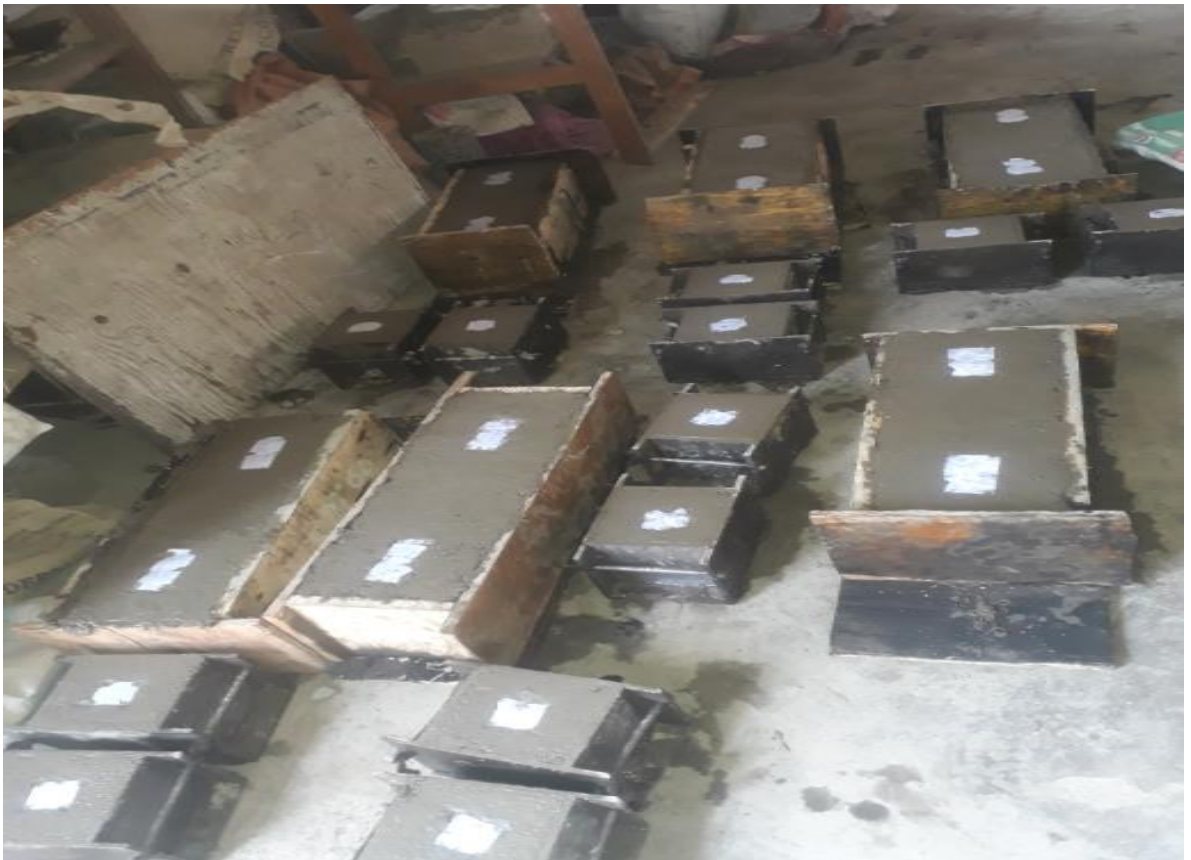
Figure C.5. Beams casted for flexural strength test
