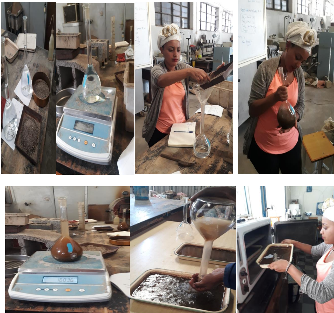
Figure 3.7. Measuring specific gravity for FA
