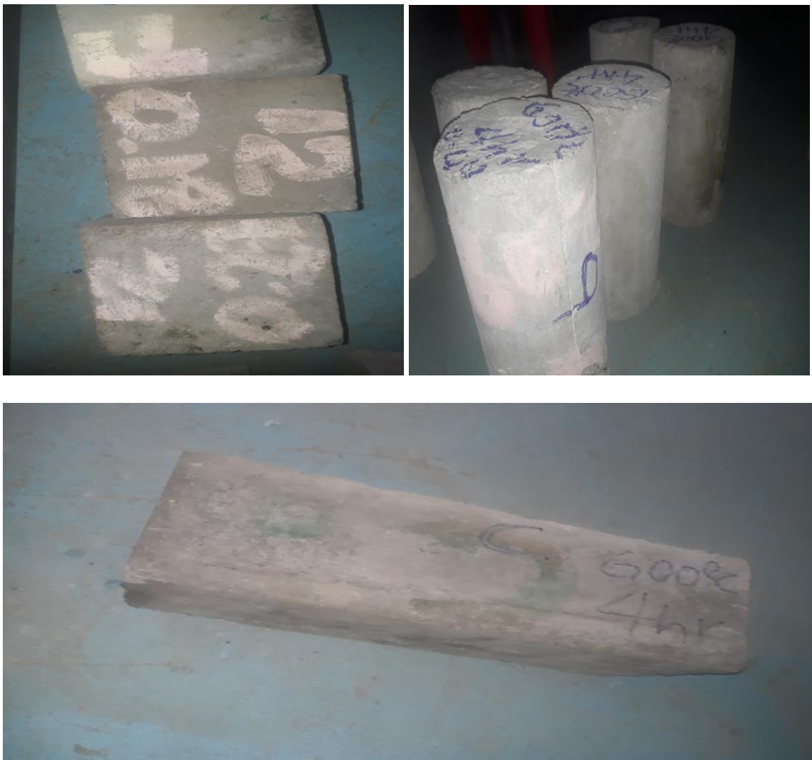
Figure 3.18. Specimen after they are exposed to fire at desired temperature One of mechanism of testing specimens exposed to fire is by air cooling system and because of lack of measuring instrument in our country all specimens after exposed to fire they are left for 24 hour before they are tested. Then all tests are conducted accordingly.
