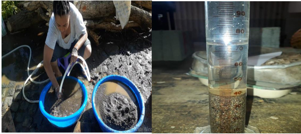
Figure 3.2. Measuring silt content of sand
