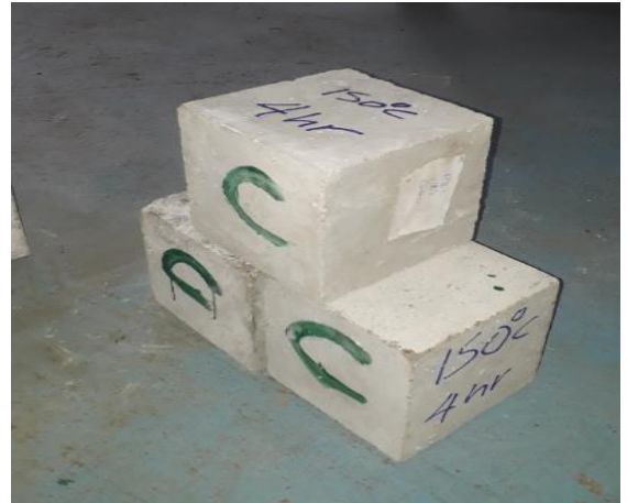
Figure 4.42. Color of specimen under 150 °C and 4hr
