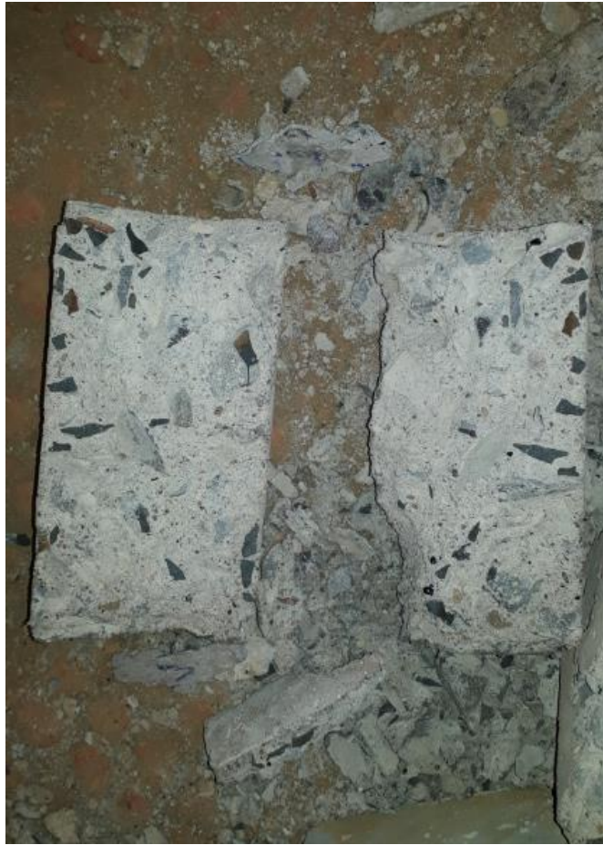
Figure C.10. Split tensile strength test of cylinders after exposed to fire
