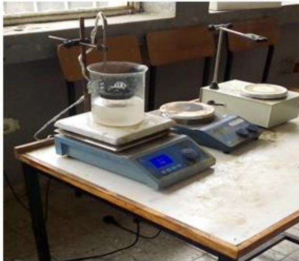
Figure 3.6 Photo shows the preparation of Zinc sulfide thin film deposition in the laboratory
