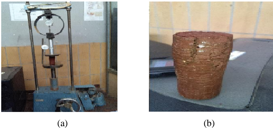
Figure 3. 4 UCS test specimens (a) during and (b) after the test
