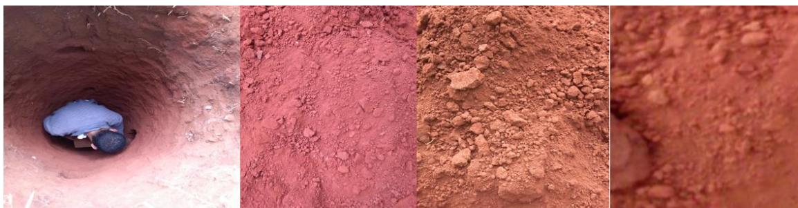
Figure 3. 3 Typical soil profile and in place soil color of the trial pits.
