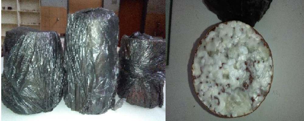
Figure 3. 2 Undisturbed soil sample covered with plastic bag and candle wax
