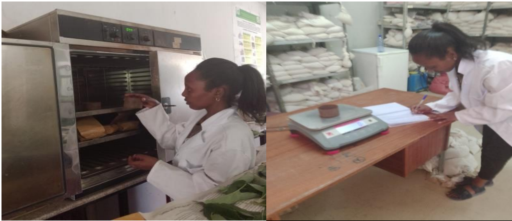
Figure 3. 8: Soil moisture determination using oven dry method.
