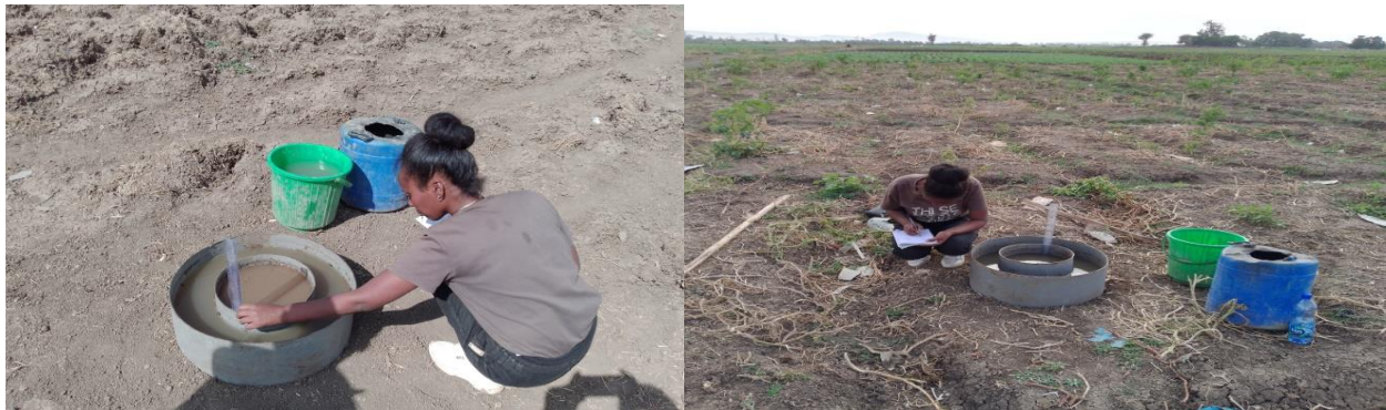
Figure 3. 9: Infiltration rate test at field level
