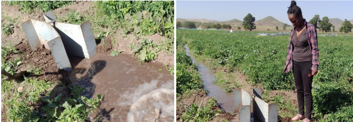
Figure 3. 10: Measurement of Field Applied Irrigation Water Using Parshall Flume
