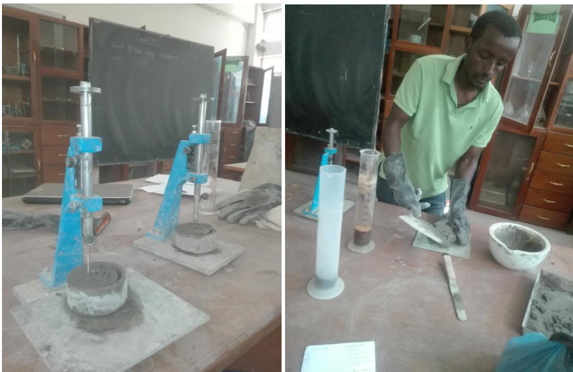
Photo 6. Consistency and setting time determination under progress using vicat apparatus
