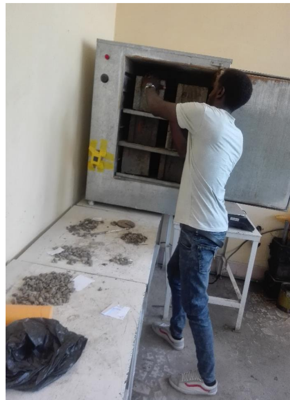
Photo 12. Immersion of blocks for Water absorption test (left), and drying HCB in oven under progress for density and water absorption test (right)
