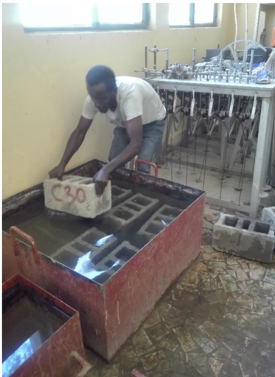
Photo 12. Immersion of blocks for Water absorption test (left), and drying HCB in oven under progress for density and water absorption test (right)
