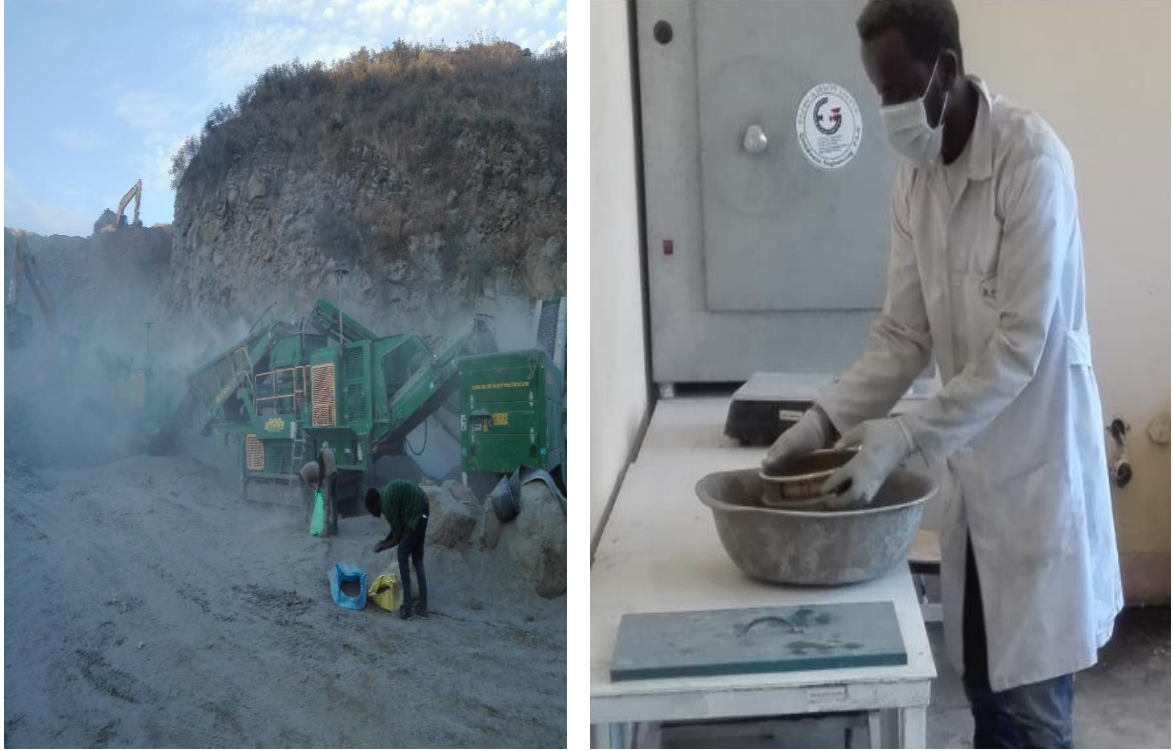
Photo 1. Crusher dust collection (left) and preparation using 150µm sieve size (right)
