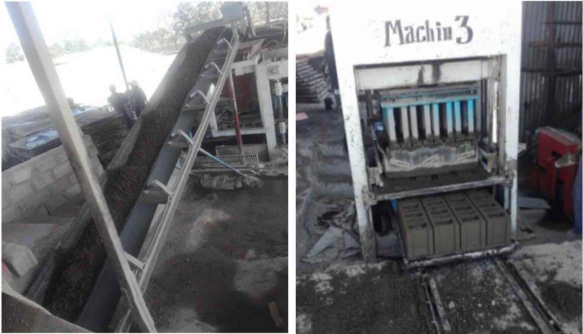
Photo 7. Conveyor belt transporting a mix to the mold (Left); HCB produced using the crusher dust and cement (Right)
