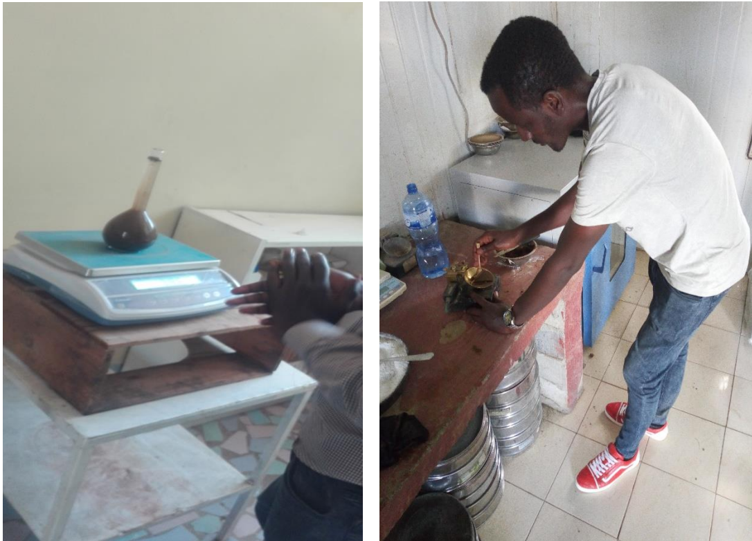
Photo 5. The specific gravity test for fine aggregate under progress (left) and plasticity index determination of BSD by Casagrande method (right)
