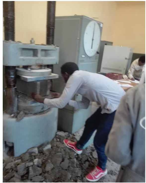
Photo 11. Arranging HCBs according to their mix code (left) and compressive strength under progress (right)
