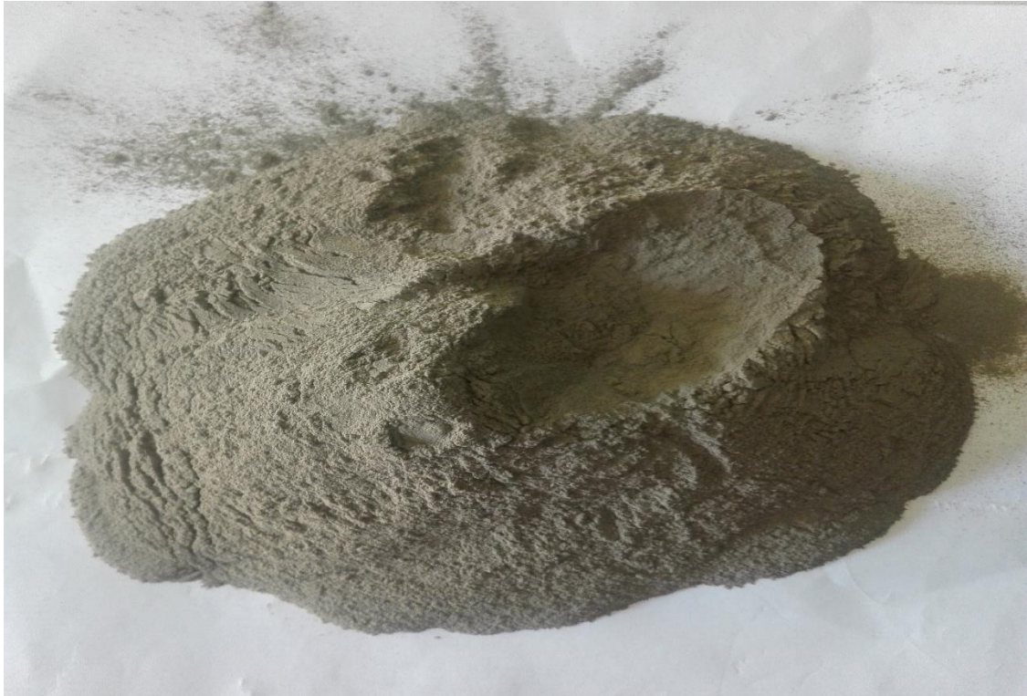
Figure 3.3 Basaltic crusher dust sample after sieving with 150 \mu m sieve (Crusher dust used for the research)
