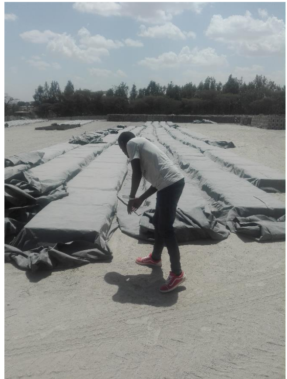
Photo 9. Fresh blocks left on wooden pallet for 1 day (Left) and Curing of blocks by covering plastic (Right)
