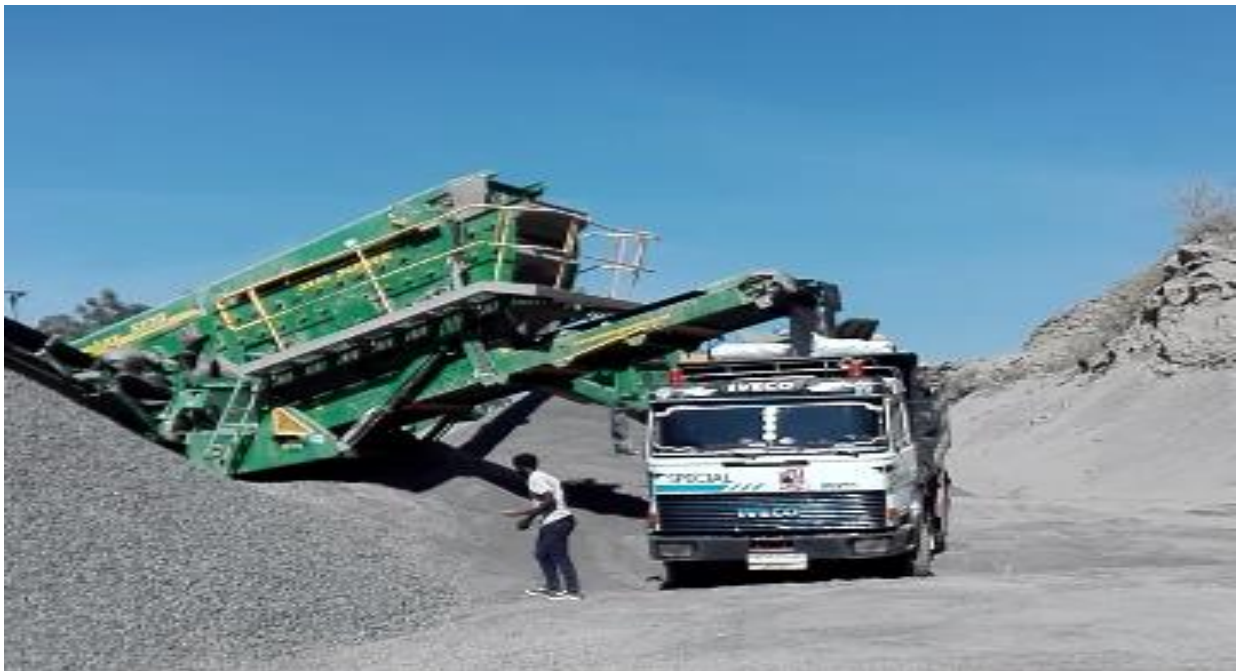
Figure 2.3 Hauling truck collecting a by-product blended with fines as a manufactured sand
