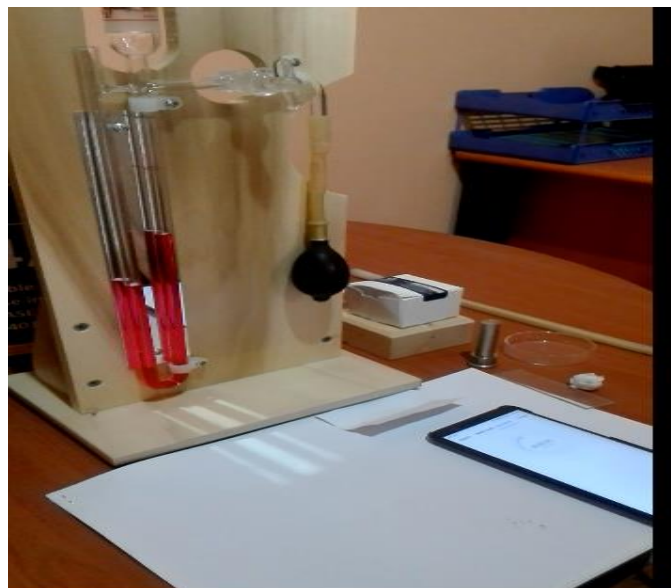
Photo 2. Fineness test under progress by Blaine air permeability apparatus
