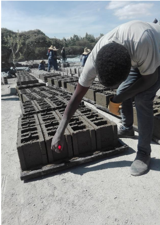
Photo 9. Fresh blocks left on wooden pallet for 1 day (Left) and Curing of blocks by covering plastic (Right)
