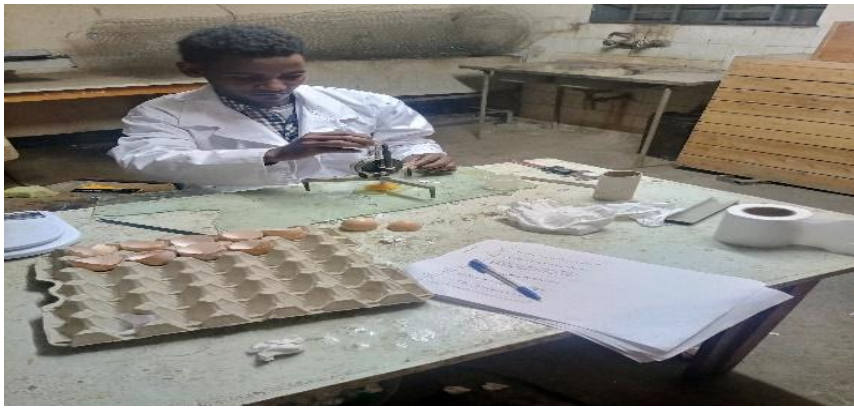
Appendix Figure 5: Measuring albumen height, yolk height, yolk diameter by tripod micrometer.
