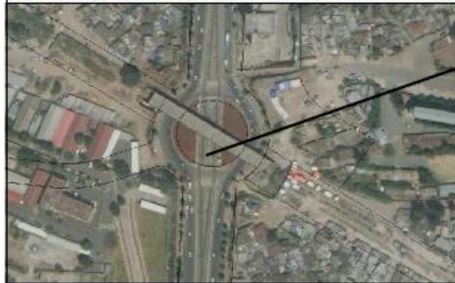
Meshualekiya level crossing This intersection has no any approach road that conflicts with the LRT line. Only vehicles that use the roundabout for changing directions. Most vehicles doesn't use the roundabout for changing directions at peak hours.
