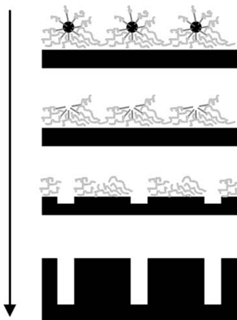
Figure 4.34 Scheme of etching semiconductor substrates, starting with gold nanoparticles containing micellar films, and followed by \text{Ar}^+ beam etching to remove the gold nanoparticles. This forms holes in the substrate with the same diameter as that of the gold nanoparticles.
