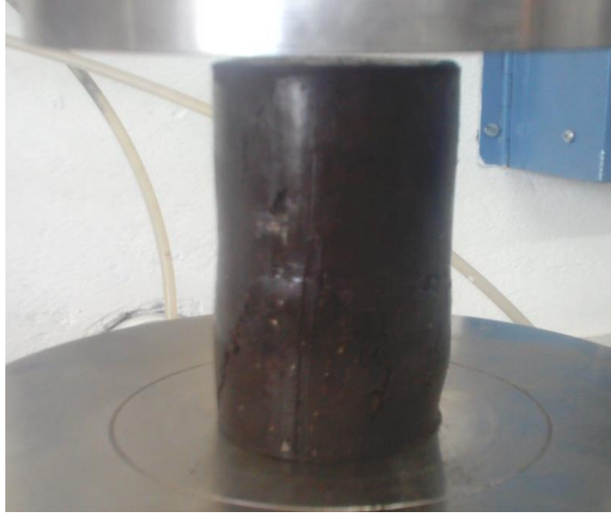
Figure 3.7: UCS Test: specimen with compression device.
