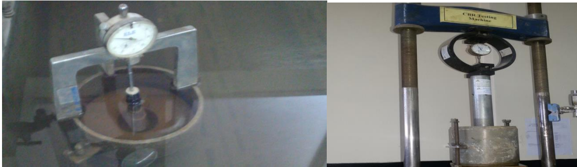
Figure 3.6: CBR Test Procedure: soaked CBR and CBR penetration.
