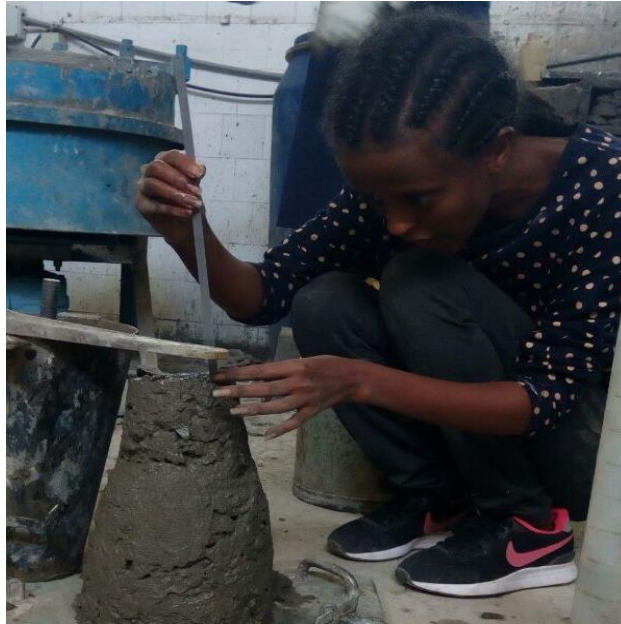
Figure 3.7: Slump test result
