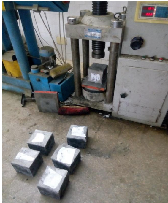
Figure 3.8: Compressive Strength Test on Compression Testing Machine
