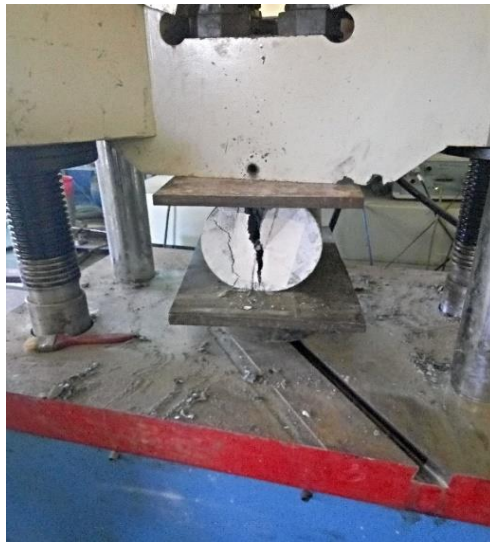
Figure 3.9: Splitting tensile strength test of concrete
