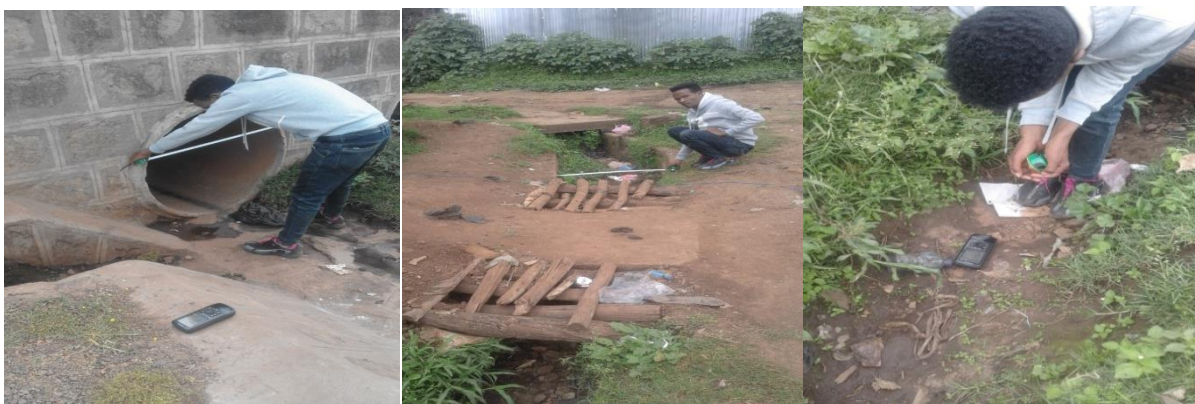
Figure 3.21: Surveying Nodes dimensions and channel cross sections by using tape meter
