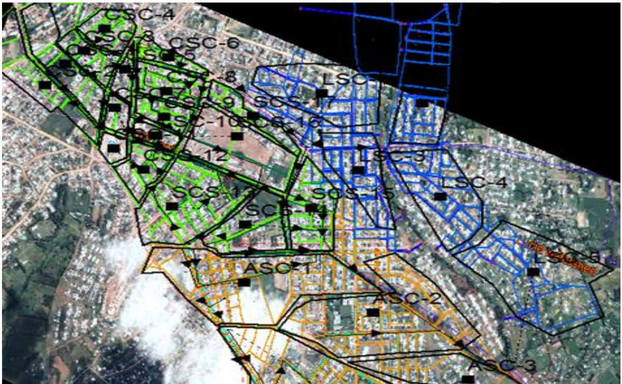
Figure 3.14: Addis sub-city City center watershed Google earth image shows the location of sub-catchments and flow direction (Source: - Google earth pro SWMM analysis).
