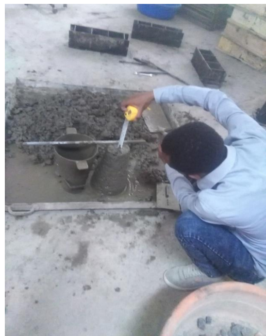
Figure F.11 Slump cone test
