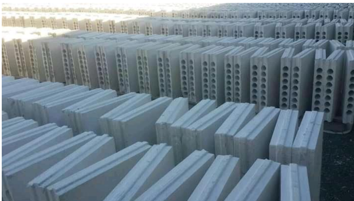
Figure 0.9 Prefab concrete blocks produced by England company in Ghana for school construction (source: Fordjour, 2015)
