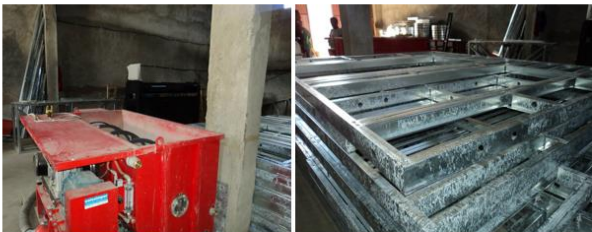
Figure 4.14 Left) high-tech steel framing machine Right) product of LGS
