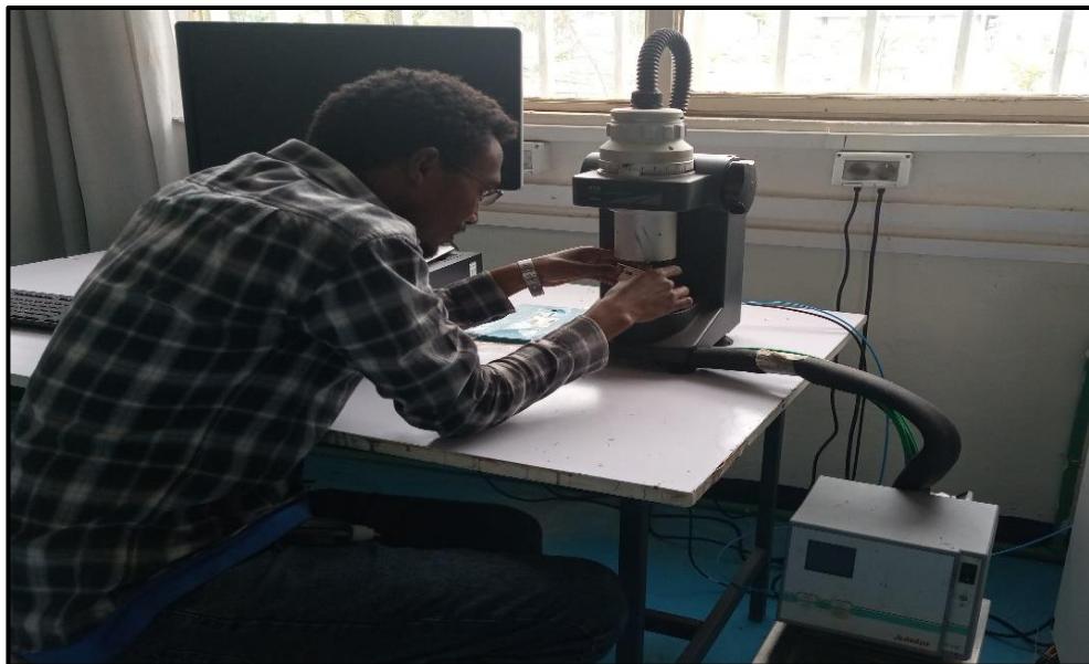
Figure 3.5 Dynamic Shear Rheometer Setup
