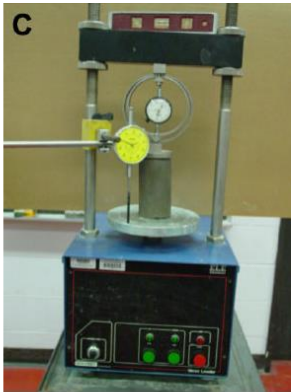
Figure 3.5 Unconfined compressive testing equipment (Reddy, 2002)
