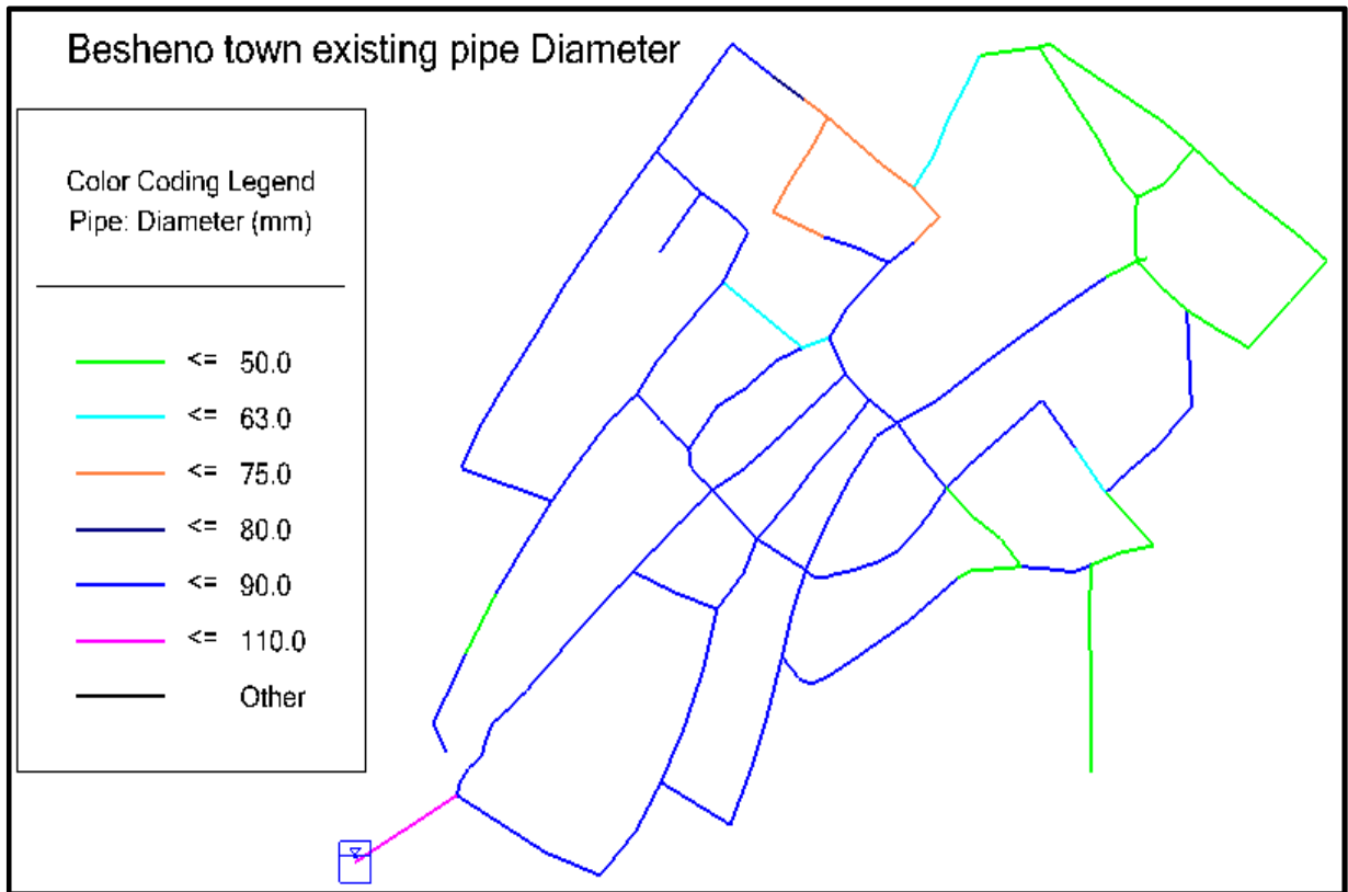
Figure 4.4: Besheno town existing pipes diameter
