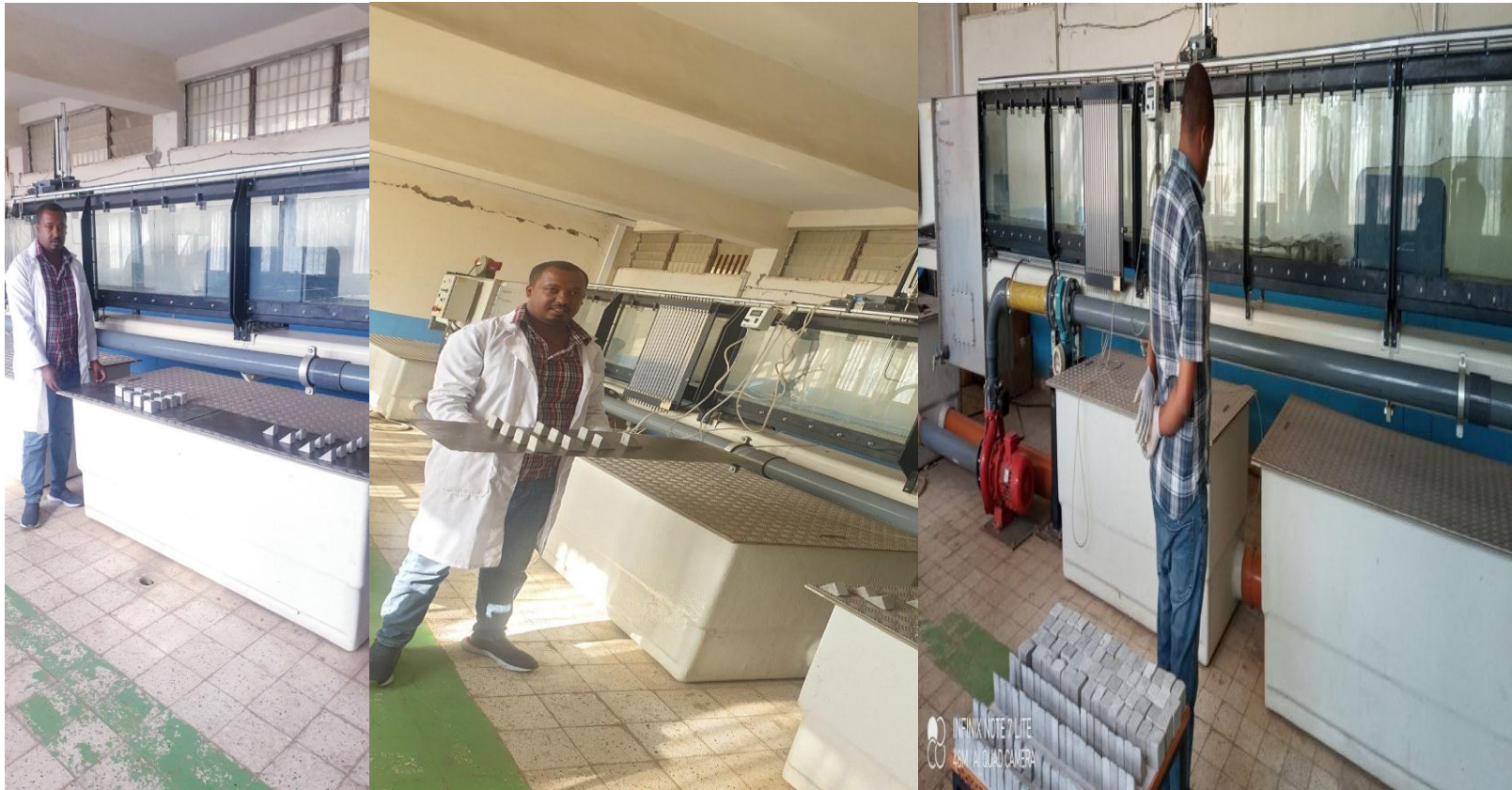
Figure B.1 Putting Baffle Block Bed in the experimental Flume
