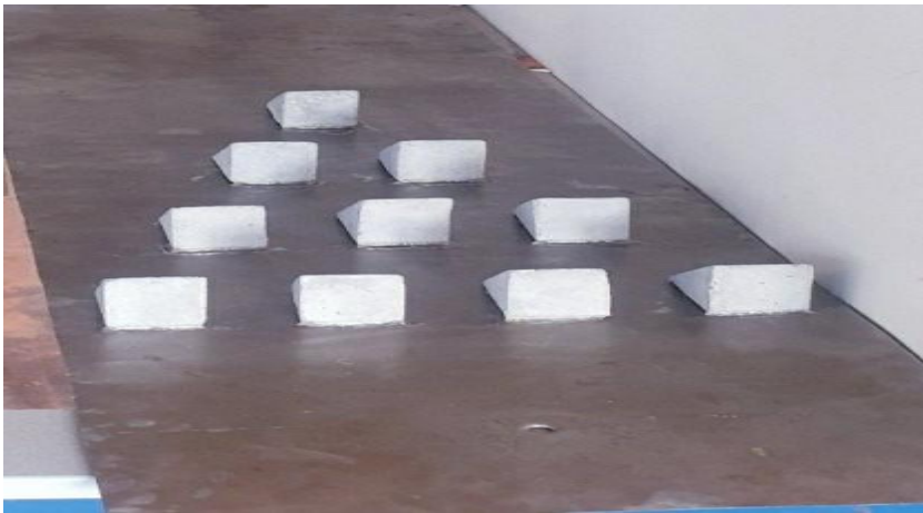
Figure 3-4 baffles block Model arrangement
