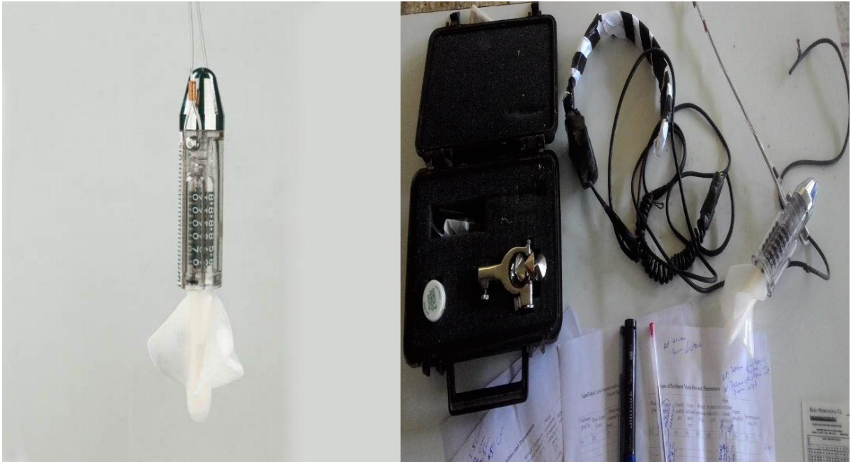
Figure 3-10 Mechanical Current Meter with accessory (Hu-IoT laboratory)
