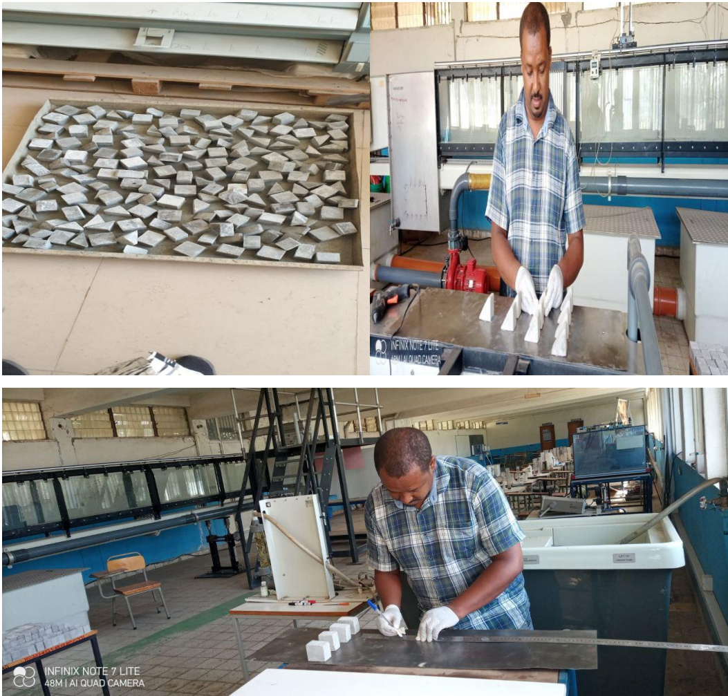
Figure 3-8 Preparation of baffle block and arrangement model
