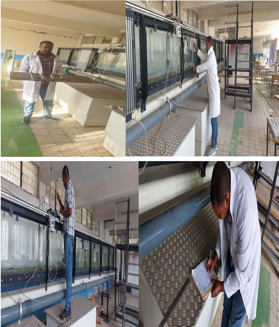
Figure 3-9 Photographs of experimental arrangement with baffle block modeling open channel flume.
