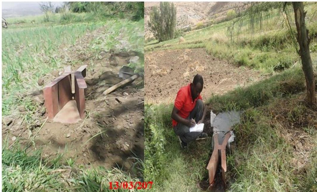
Figure in appendix 4: Discharge measurement at field application using parsshall flume
