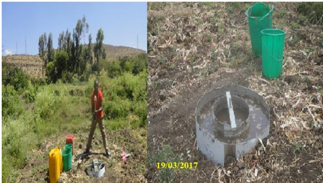
Figure in appendix 2: During infiltration measurement at field
