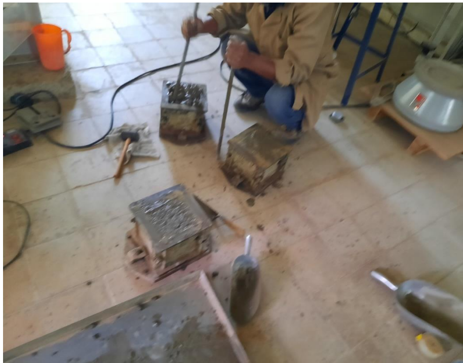
Figure AN. E-14: Concrete casting
