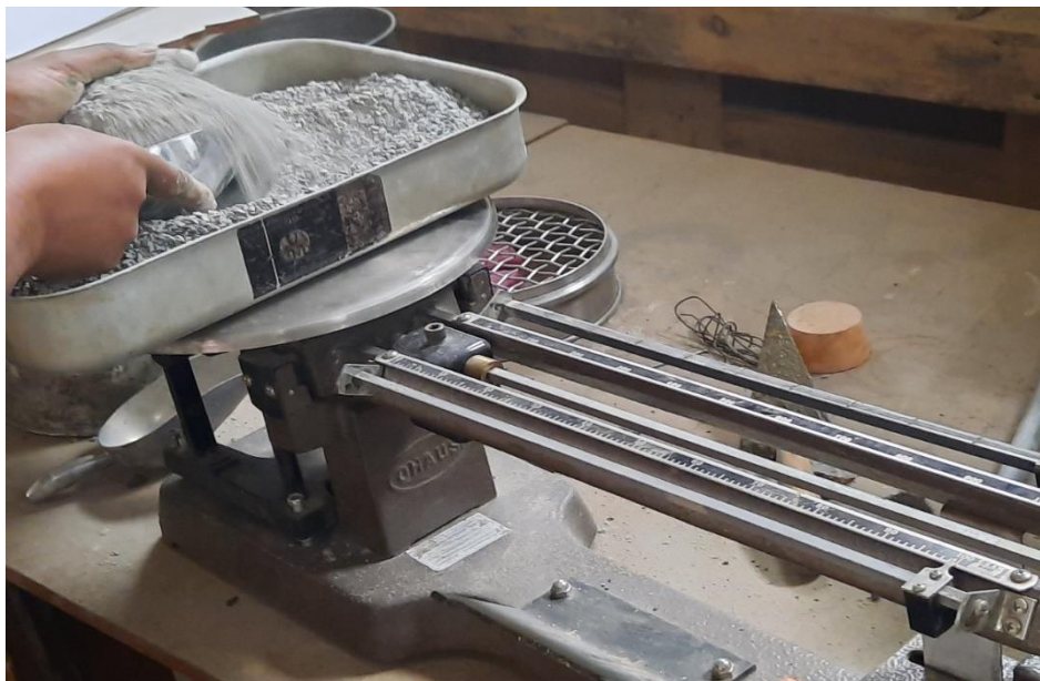
Figure AN. E-9: Weighting river sand
