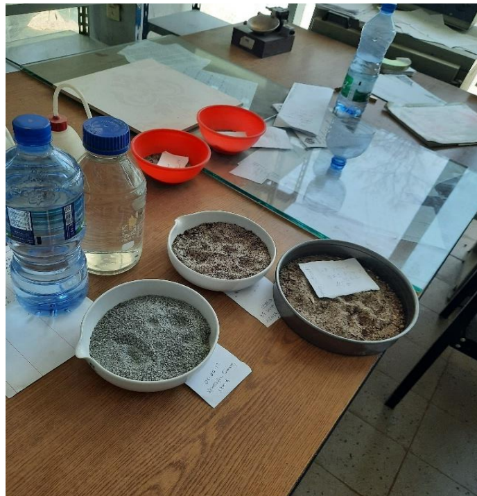
Figure AN. E-6: River sand and stone dust to determine specific gravity
