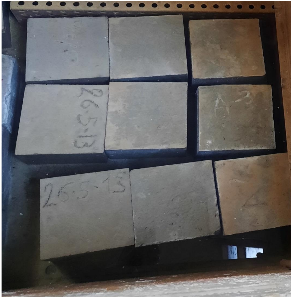
Figure 3.17: Immersion to test for water absorption
