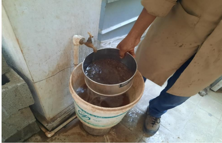
Figure AN. E-5: Washing of sand
