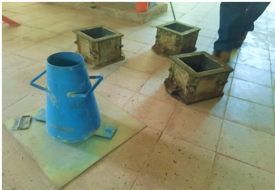
Figure 3.10: Preparing of molds to cast concrete
