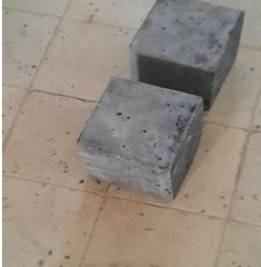
Figure AN. E-16: Water Cured concrete
