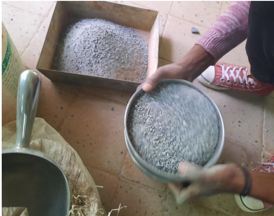
Figure 3.6: Preparing quarry dust for physical property test
