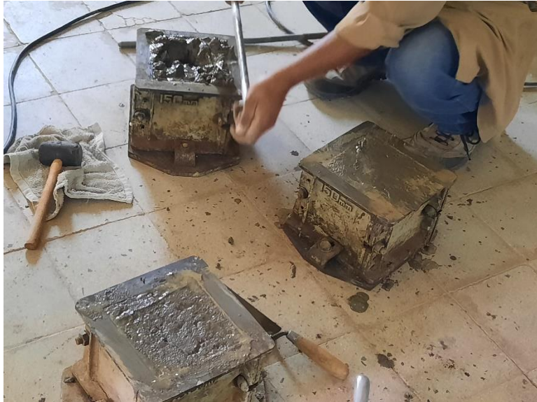
Figure 3.11: Casting and compacting of concrete
