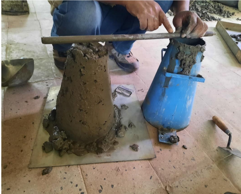
Figure AN. E-13: Preparing for slump test
