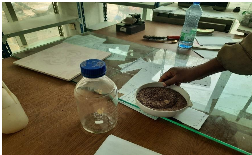
Figure 3.4: Preparing sand to test for physical properties
