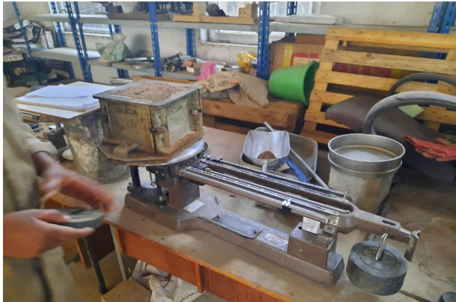
Figure AN. E-9: Weighting river sand
