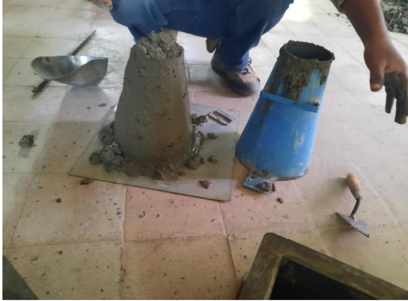
Figure 3.12: Removing mold for slump test
