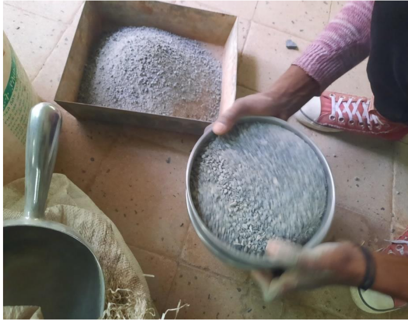
Figure AN. E-3: sieving of stone dust
