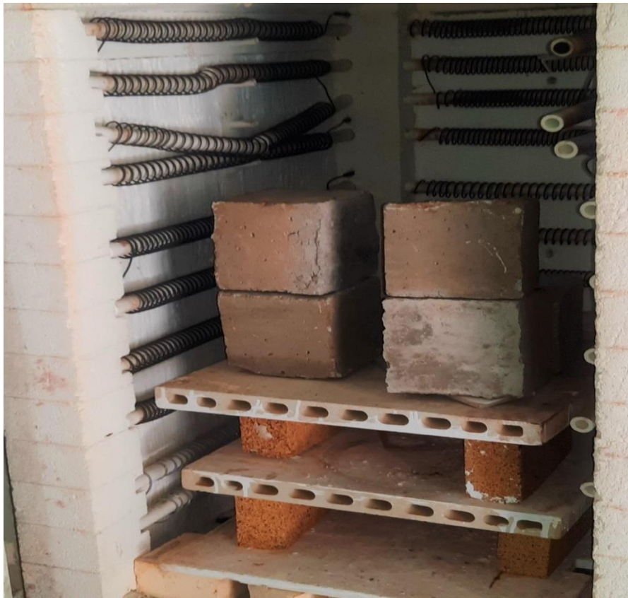
Figure 3.16 Burning of concrete cubes
