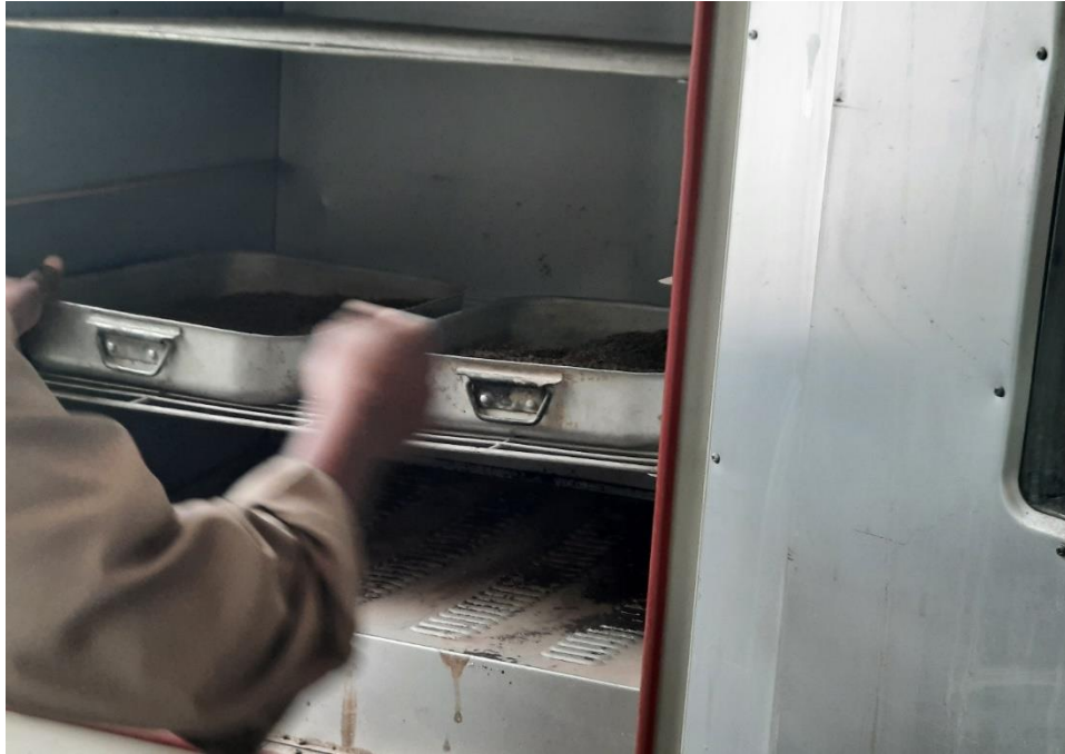
Figure AN. E-11: oven drying (River sand, Stone dust and coarse aggregate)
