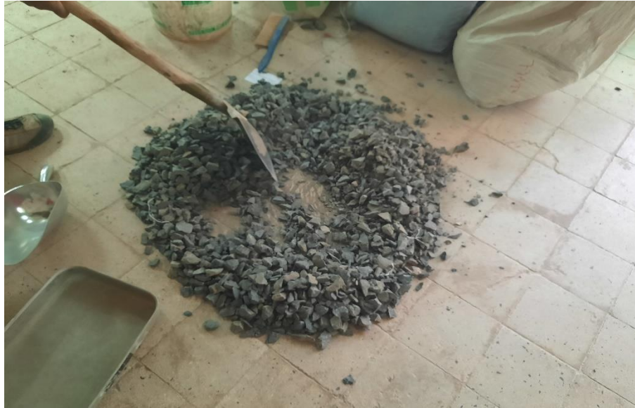
Figure 3.1: Preparing coarse aggregate to test for its property
