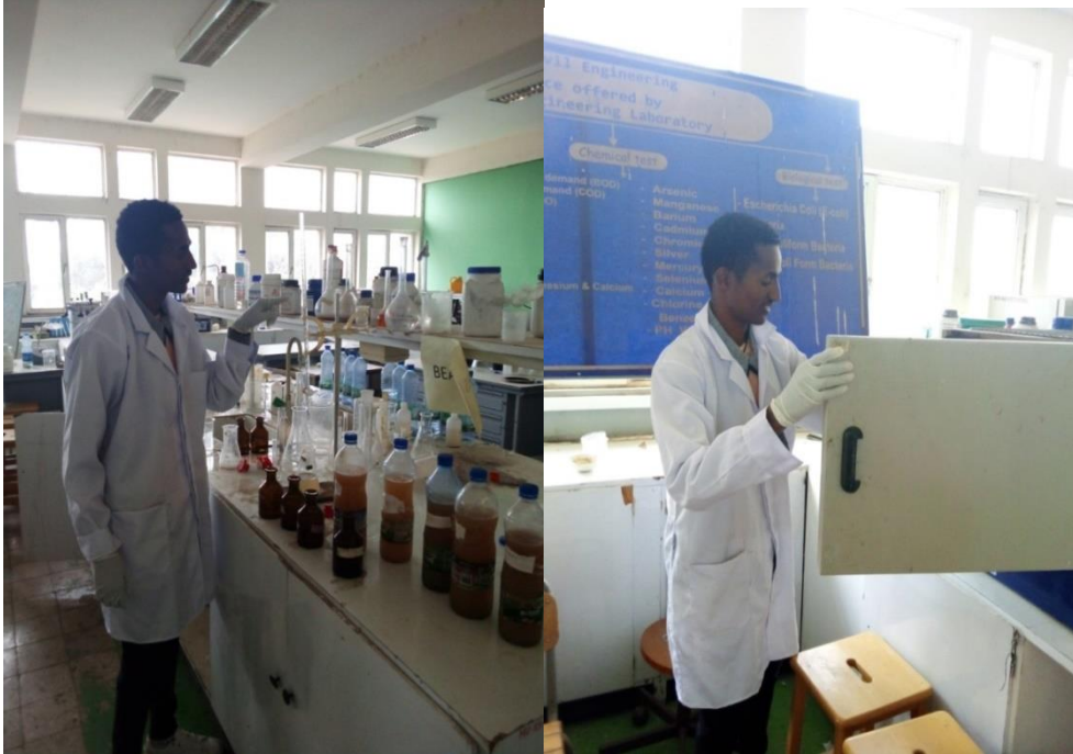
Image shows measuring the DO by titration and insert sample in oven for determining TSS
