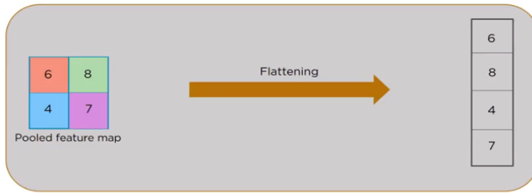
Figure 10: Sample Flattening Layer
