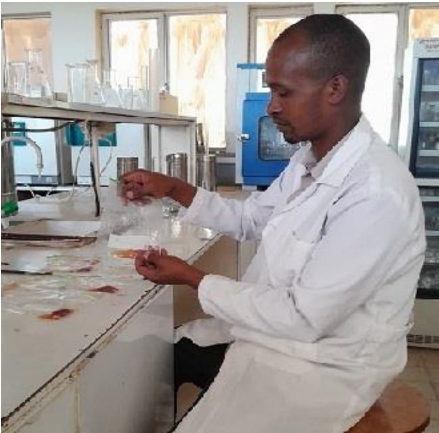
4. Massaging of beef sample with buffered peptone water in a plastic bag
