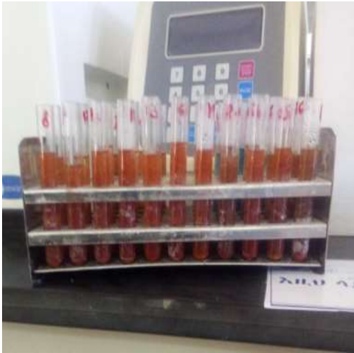
Annex 6: (a) mixture of benedict solution and hydrolyzed sample (b) heated mixture in water bath (c) Absorbance reading by spectrophotometer.
