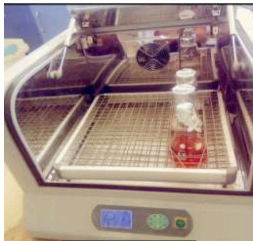
Annex 9: (a) Sample ready for fermentation (b) Fermentation in shaking incubator
