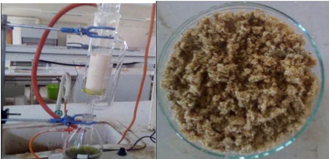
Annex 2: (a) Soxhlet extraction setup (b) Extractive free sampe
