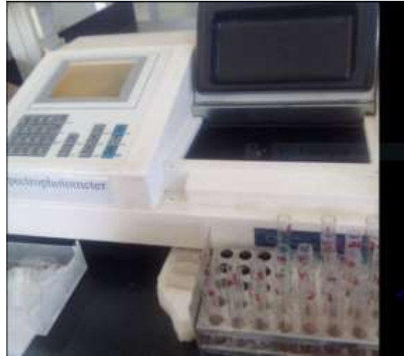
Annex 6: (a) mixture of benedict solution and hydrolyzed sample (b) heated mixture in water bath (c) Absorbance reading by spectrophotometer.
