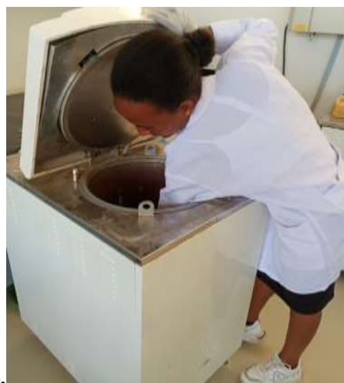
Annex 4: (a) Sample with diluted H 2 SO 4 solution ready for hydrolysis (b) hydrolysis sample solution in autoclave.
