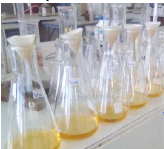
Annex 4: (a) Sample with diluted H 2 SO 4 solution ready for hydrolysis (b) hydrolysis sample solution in autoclave.
