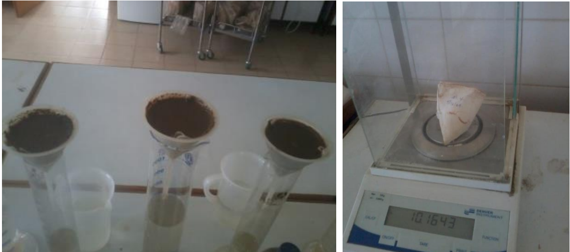
Figure 3-4 sediment filtering and weighing in a laboratory.
