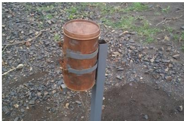
Figure 3-2 Manual rain gauge in the watershed
