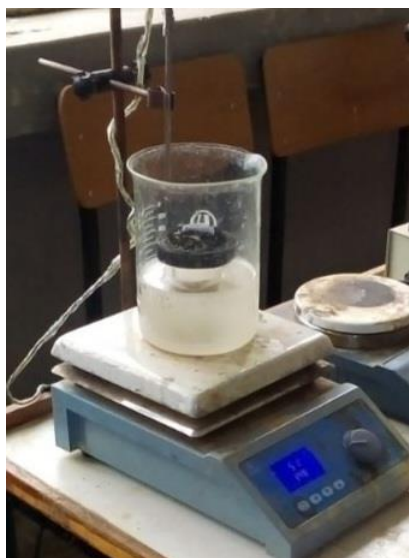
Figure.3.2: Deposition processes of zinc sulfide thin films.
