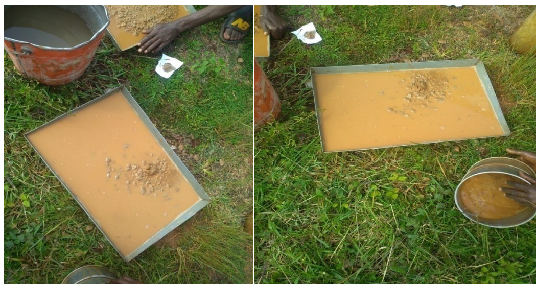
Figure.4.9 Preparation of weathered yellowish laterite for wet sieving
