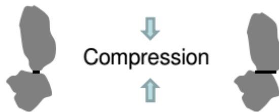
Figure 4.28 Elastic increase in the contact area between the particles due to compaction source : (Jan, 2011).
