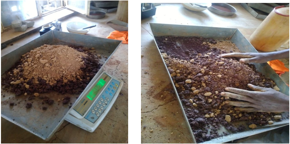
Figure 4.12 Mixing cinder material with weathered yellowish material
