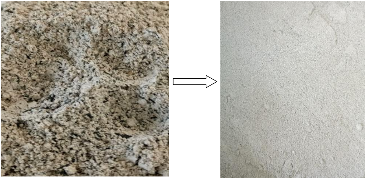
Figure 3-2 CHA, after burning (a) and, after grinding and sieving (b)
