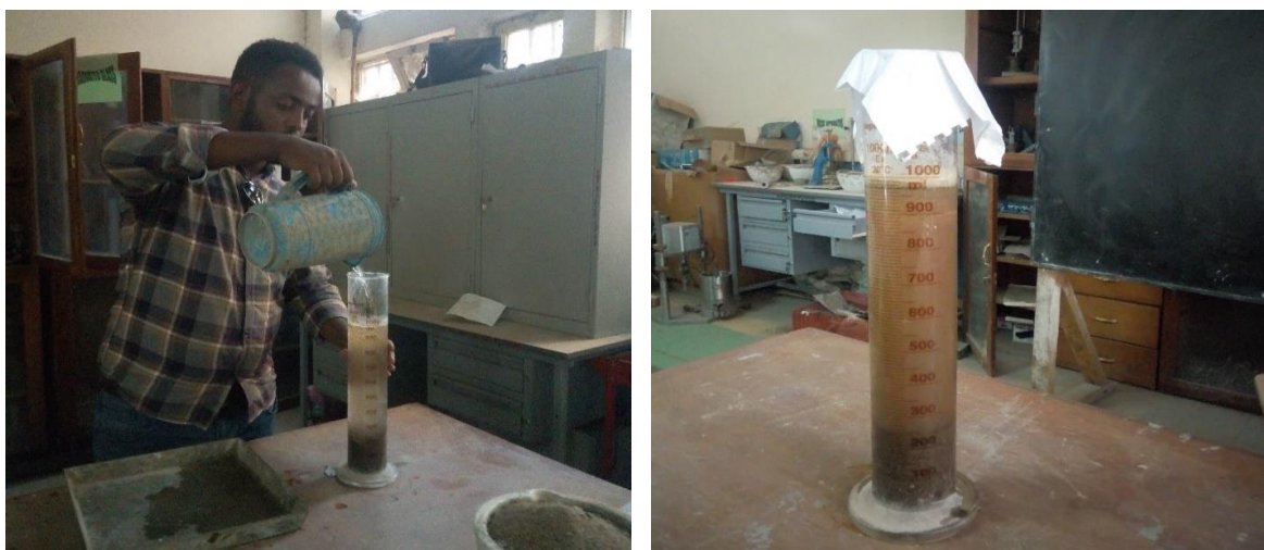
Figure 3.2 Silt content test for a fine aggregate
