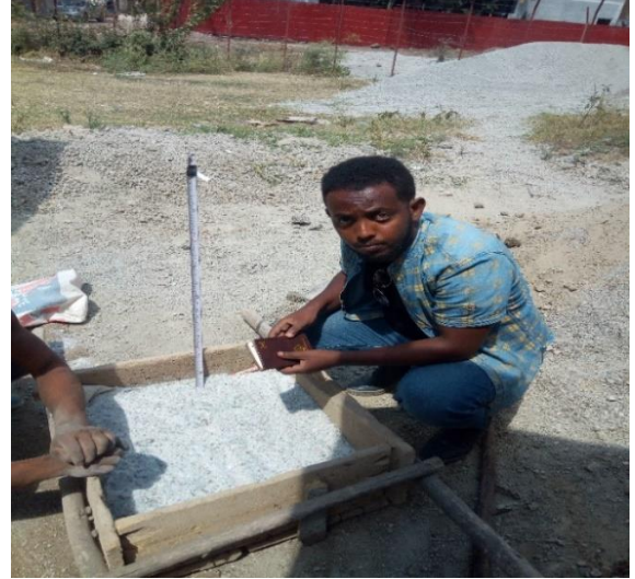
Mixing the crushed waste glass with concrete block making materials
