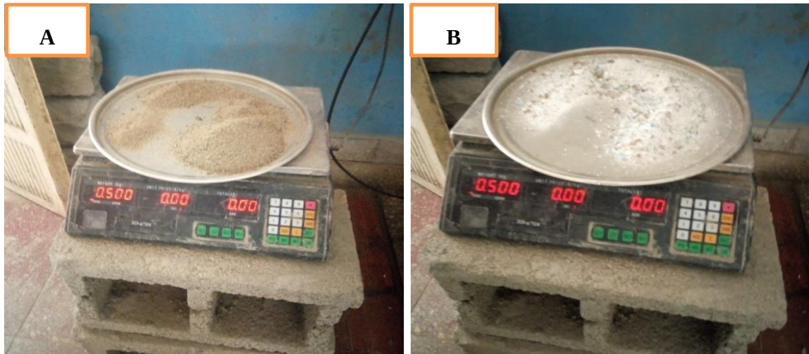
Figure 3.3 The sieve samples of 500g (A) for fine aggregate and (B) for CWG
