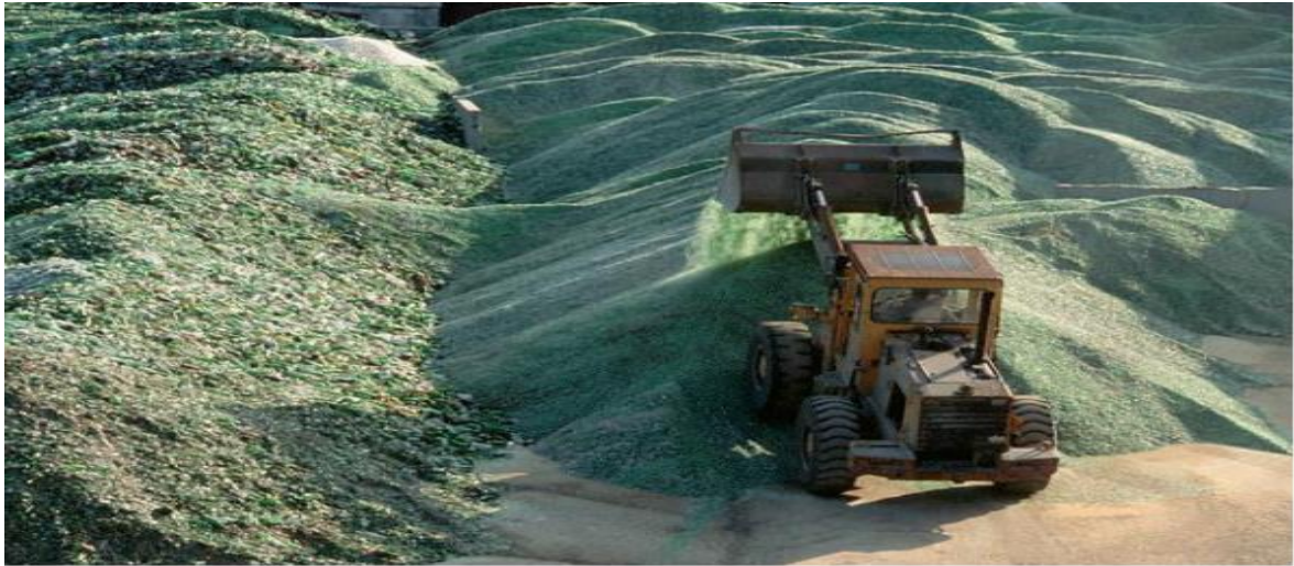
Figure 2.3 A sample of recycled glass waste cullet stockpile in West Virginia (1993) (Source: Rajabipour et al., 2012).
