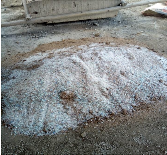
Mixing the crushed waste glass with concrete block making materials
