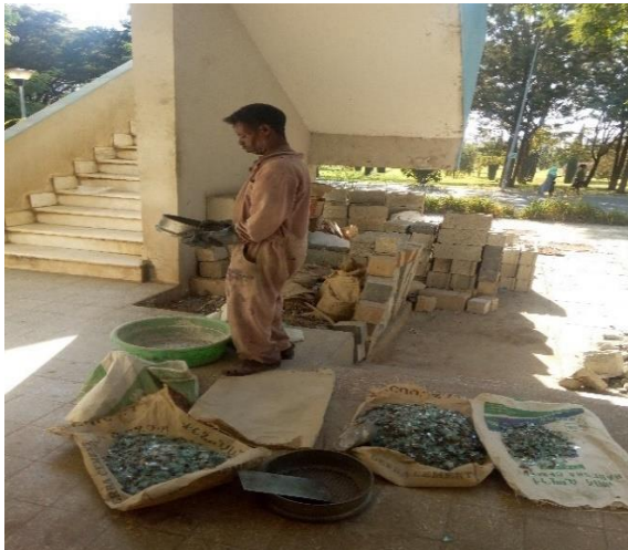
The crushed glass glasses sieved by ASTM 4.75mm into fine aggregate sizes
