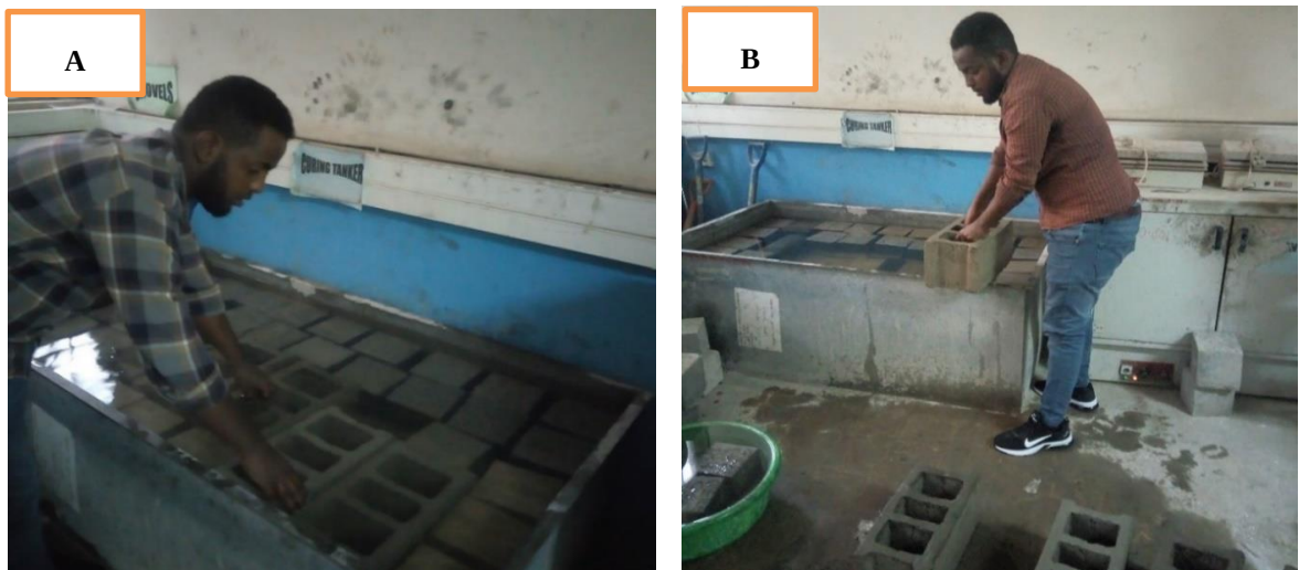
Figure 3.6 The water absorption tests (A) immersed in water and (B) suspended from water
