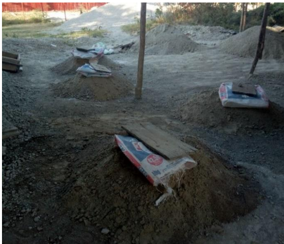
The crushed waste glass preparation mix for 10%, 20%, and 30% replacements
