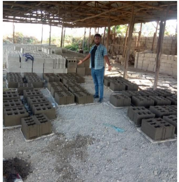
The produced hollow concrete blocks size 20*20*40 cm
