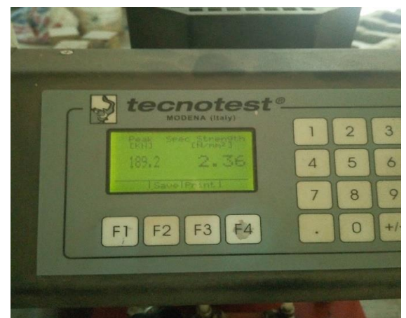
The compressive strength test machine and result
