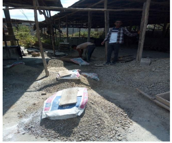
The crushed waste glass preparation mix for 10%, 20%, and 30% replacements
