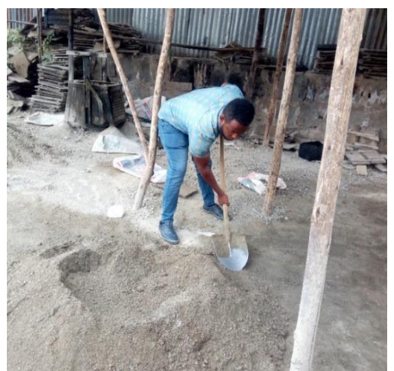
The crushed waste glass mixing for 10%, 20%, and 30% replacements
