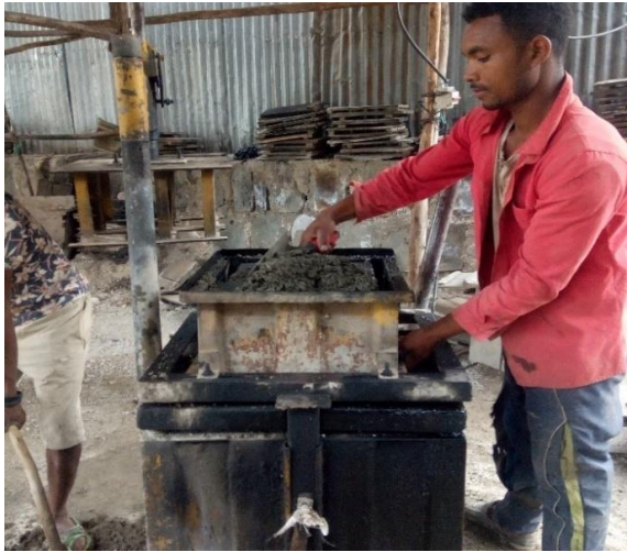
The operator making block to the size of 20*20*40 cm through manual machine
