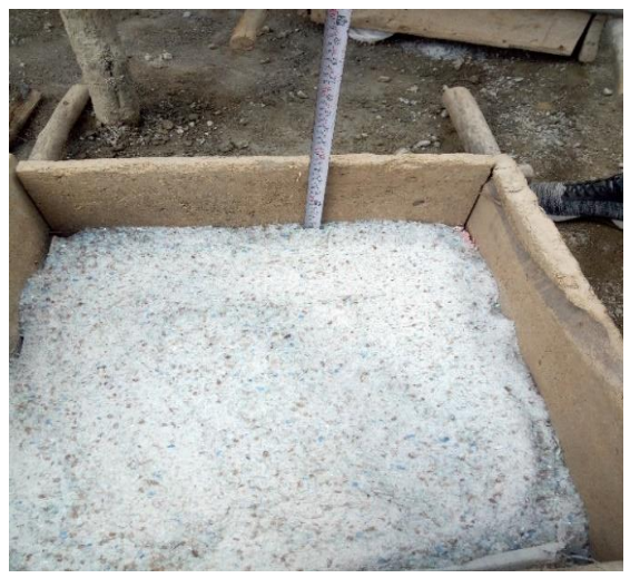
Measuring the volume of box and add the required percentages of CWG replacement
