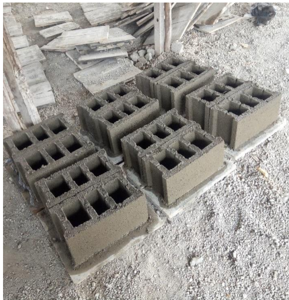
The produced hollow concrete blocks size 20*20*40 cm
