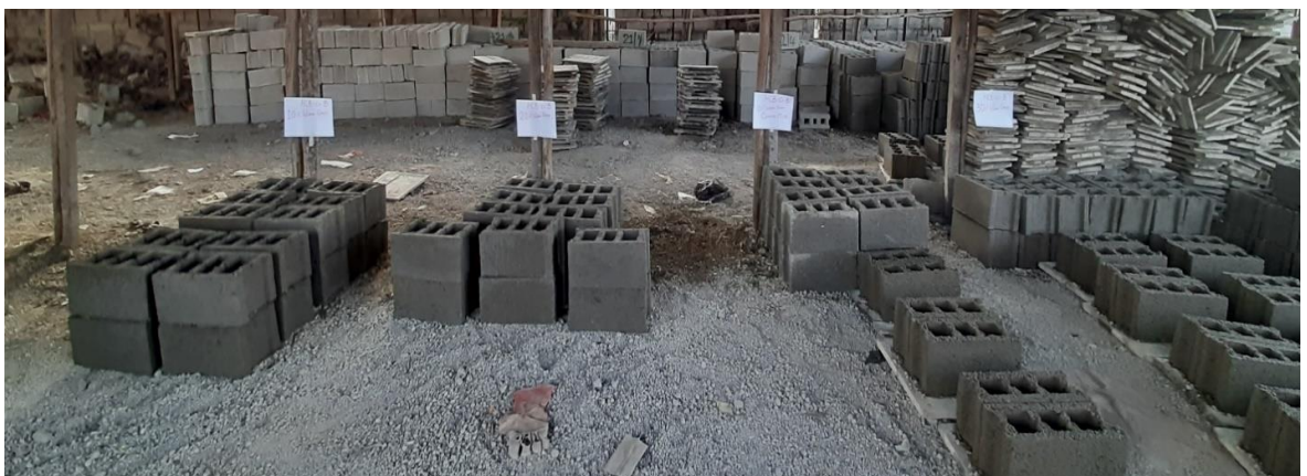
The produced hollow concrete blocks size 20*20*40 cm for 0,10,20, and 30% replacements
