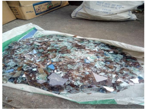
Manually crushed waste glasses
