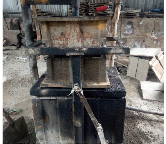
The operator making block to the size of 20*20*40 cm through manual machine
