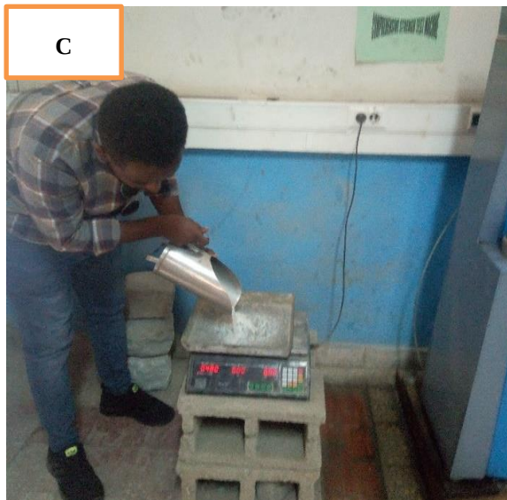
Figure 3.4 Specific gravity test A and B for fine aggregate, C and D for CWG
