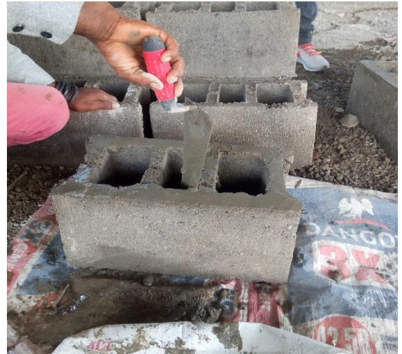
Making the block contact surfaces, with the testing machine, of each sample capping with 1:1 mortar of 2 to 3mm thickness.
