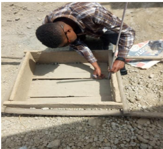
Measuring the volume of box and add the required percentages of CWG replacement
