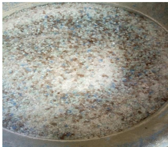
The crushed glass glasses sieved by ASTM 4.75mm into fine aggregate sizes
