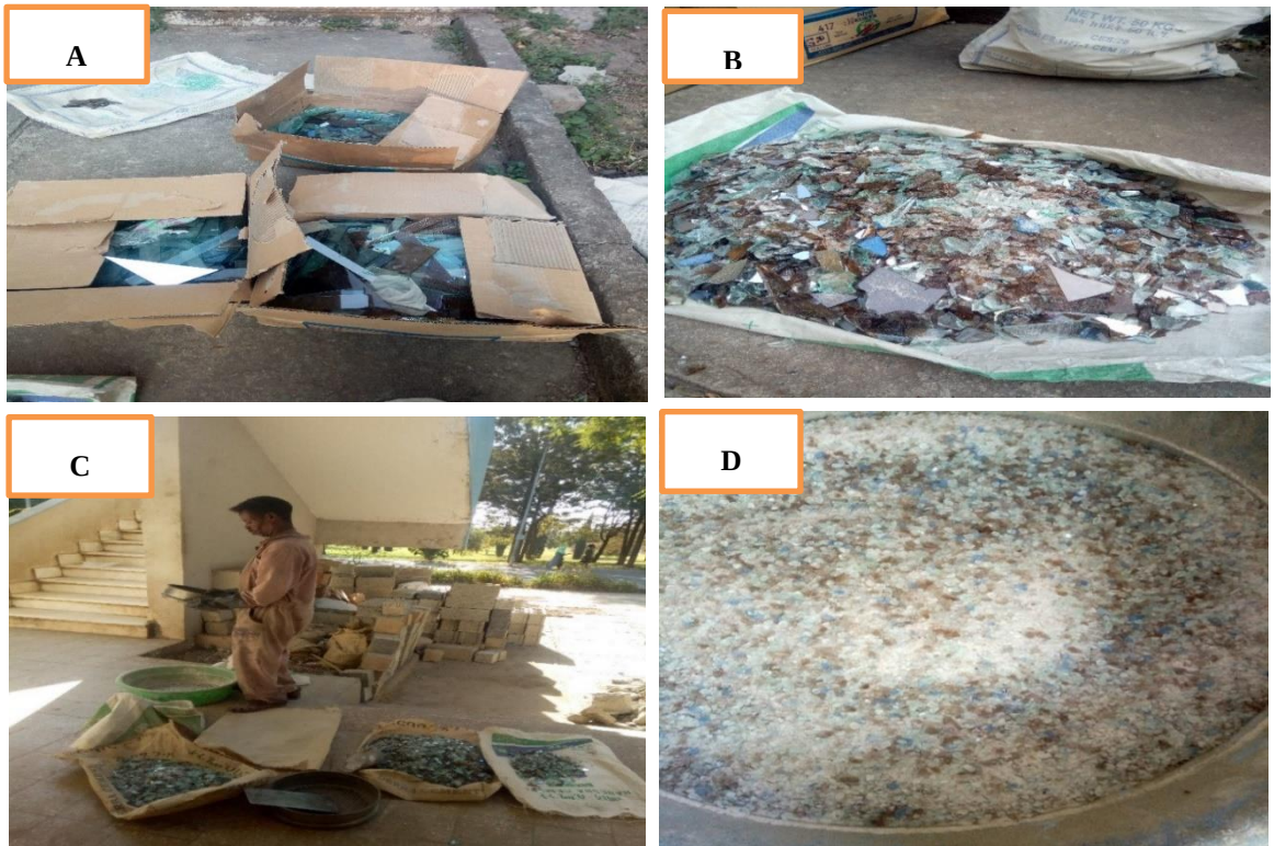
Figure 3.1 (A) CWG which are collected from waste dumping areas, (B) ready for crushing, (C) sieved by ASTM 4.75mm and (D) the sieved glass into the size of fine aggregate.
