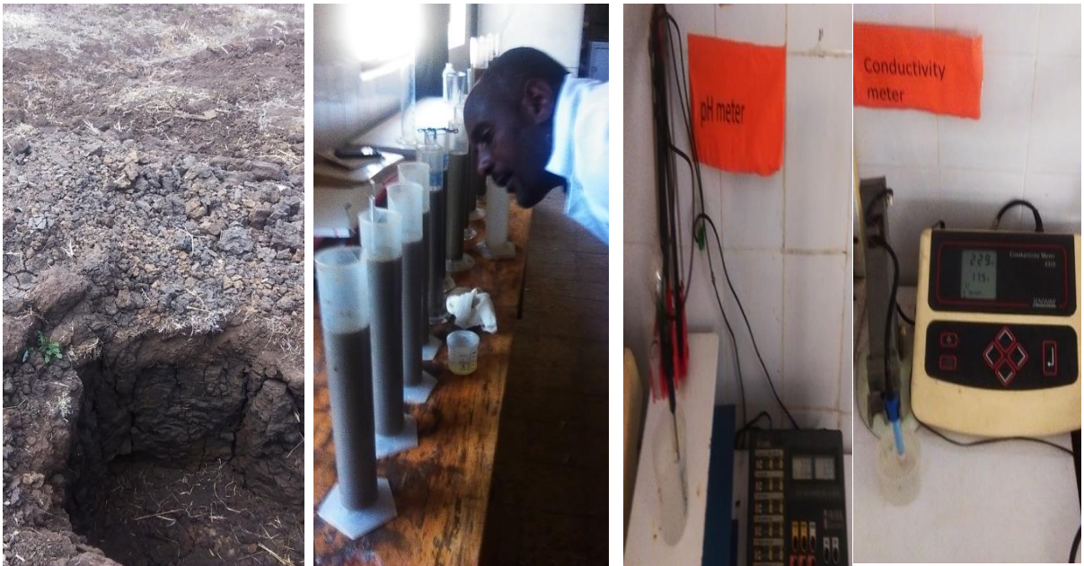
Appendix Figure 6. Soil profile pit and texture reading
