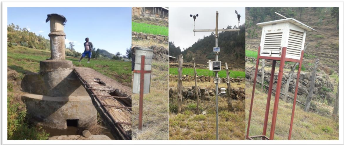
Appendix Figure 1. Hydro-sediment guage (left) and weather station (right) of Maybar watershed
