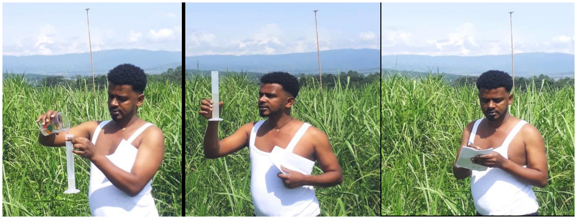
Figure 3.6 Photo during measuring catch can water volume with graduated cylinder
