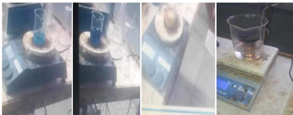
Figure 3.4: Steps of Cadmium copper oxide color change during deposition process.
