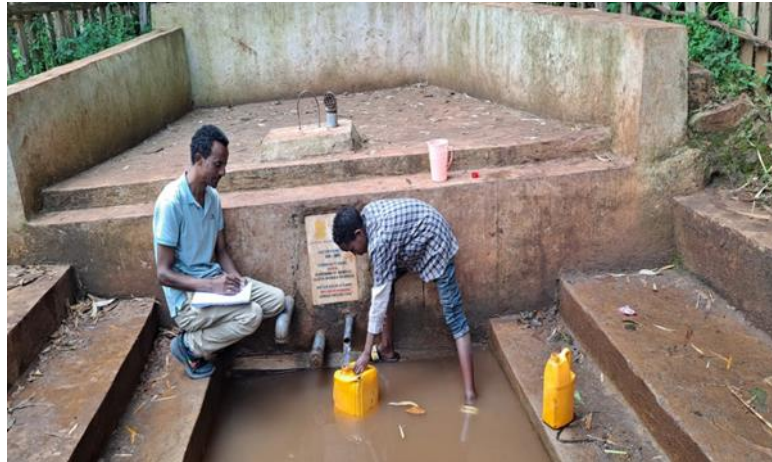
Figure 4.2 Measuring yield of spring at Gordama village
