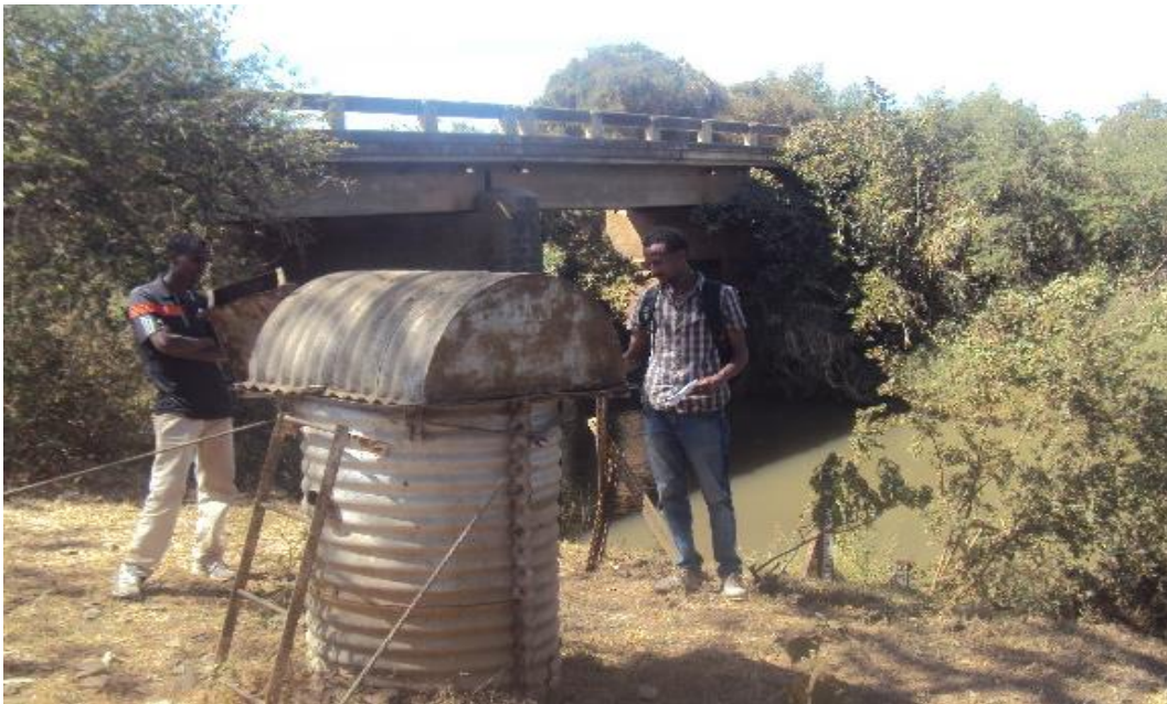
Figure 11: Discharge gauge station of Andasa River, near Andasa town
