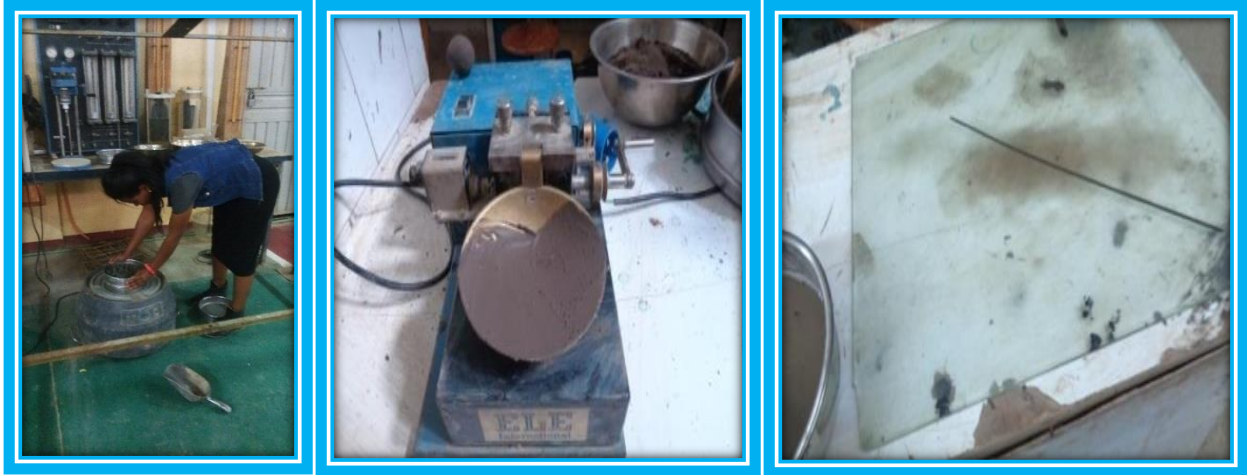
Figure 3.10: Procedures of Atterberg limit test for clay material.
