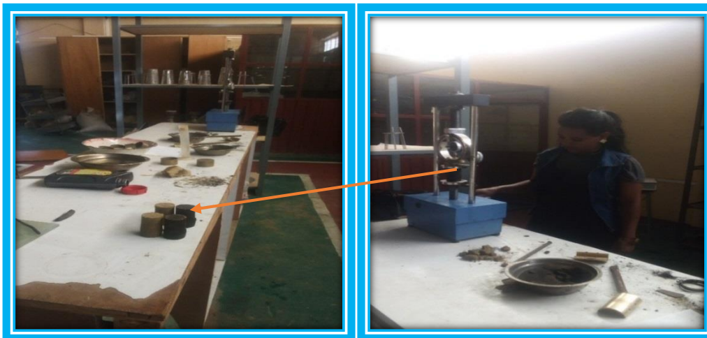
Figure 3.11: Procedures of Unconfined compression test for clay and shell material.
