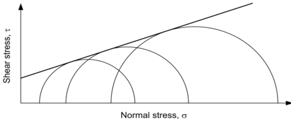
Figure 3.12 Over-stressing due to the increment of pore-pressure:
