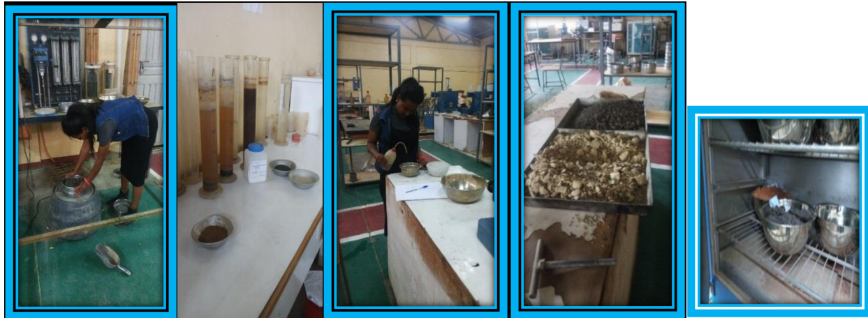
Figure 3.9: Procedures of sieve analysis for shell and Clay material.
