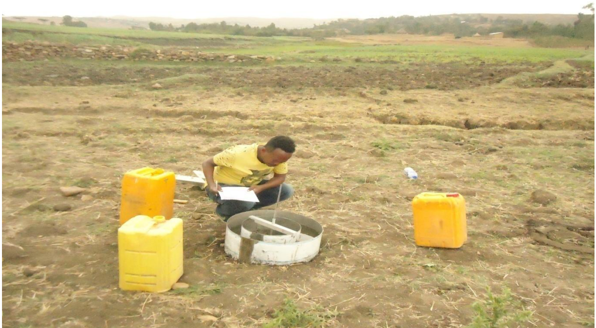
Appendix Figure 6: Measuring of Infiltration Rate using Double Ring Infiltrometer
