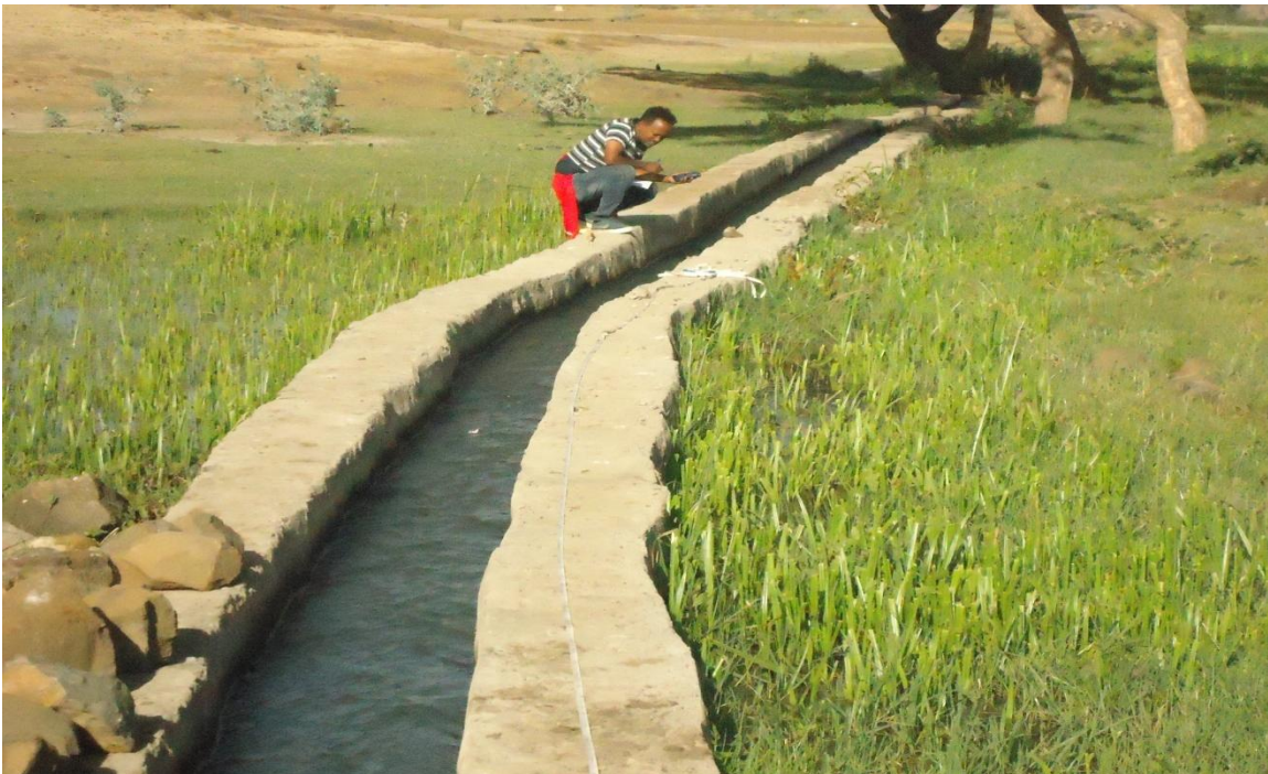
Appendix Figure 2: Measuring of discharge at the main canal using a float method.
