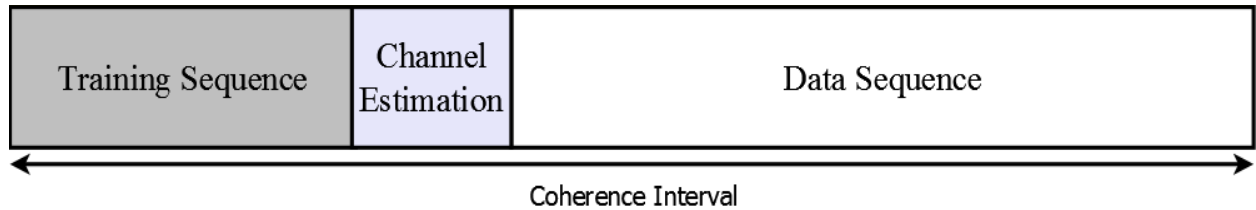
Figure 3.16: Time interval structure in pilot-based channel estimation systems [50]
