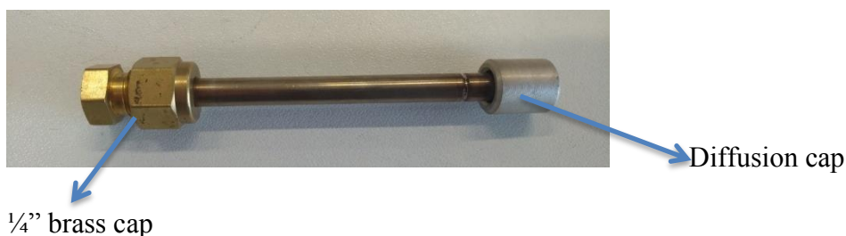
Figure 2.2. Axial passive VOC sampler (stainless steel sorbent tube)
