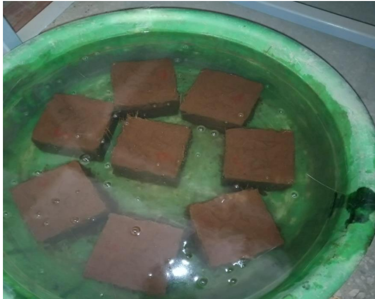
Figure (3.3) : Soaking bath to know water effect on blocks
