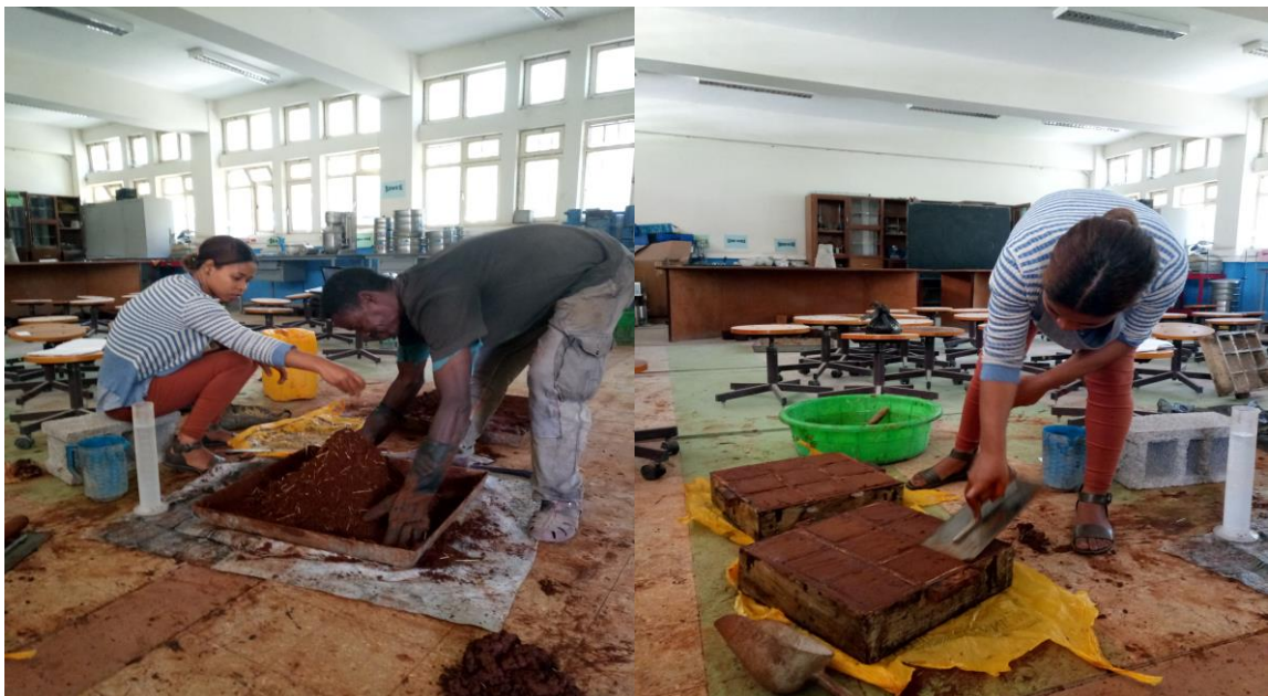
Figure (3.2) Preparing the past and the specimen
