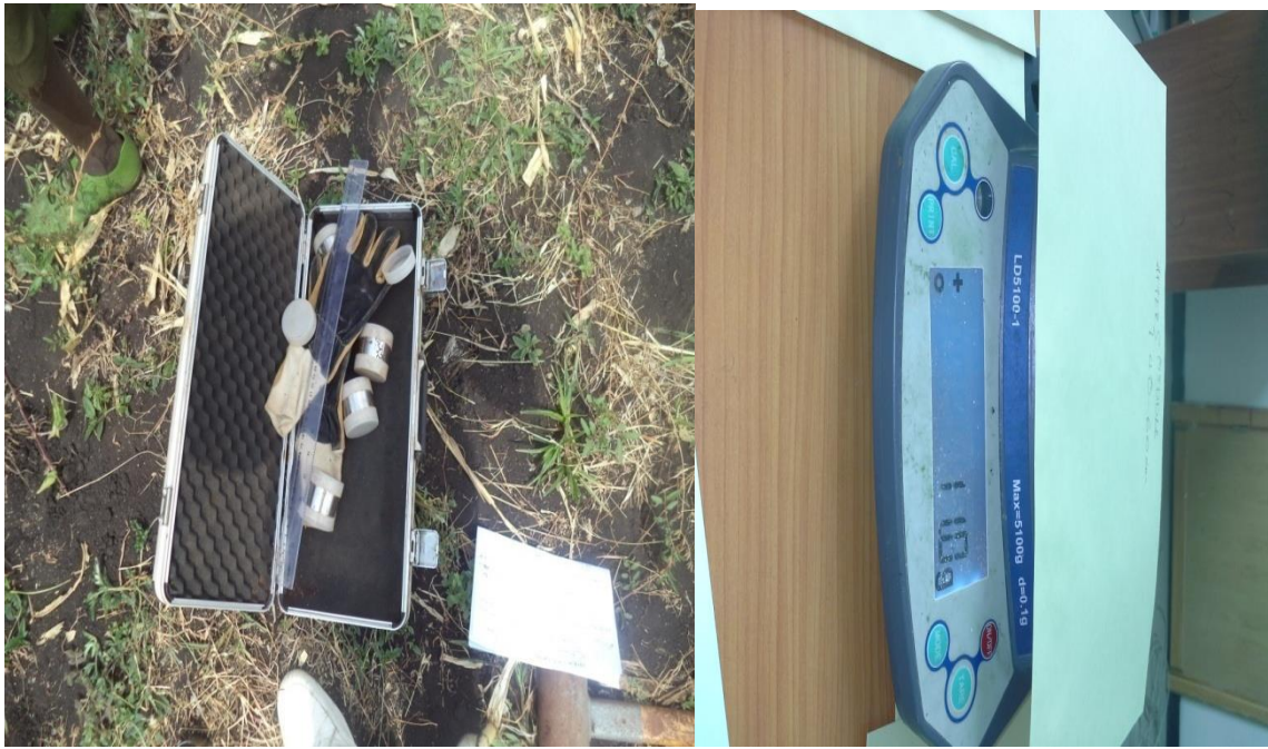
Figure 3. Core sampling auger and measuring weight of soil
