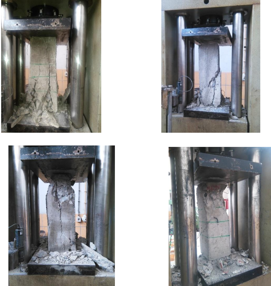
Figure 4. 10 Failure form of b; crushing failure near at the end
