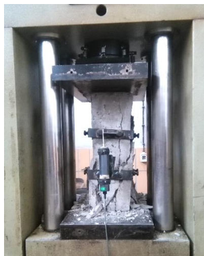
Figure 4. 14 LVDT with gauge length 165mm
