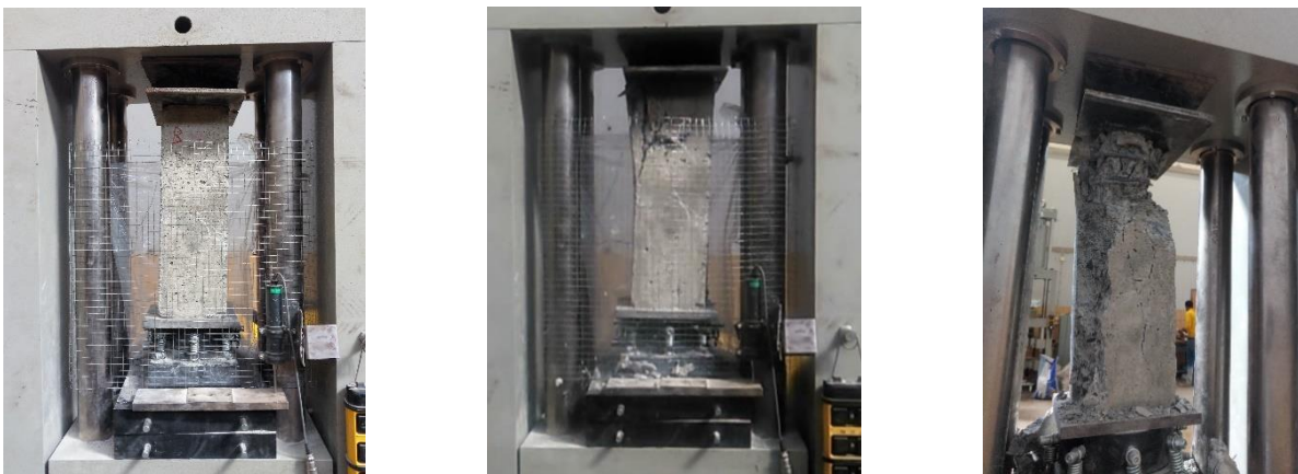
a) Before test b) surface, inclined crack and cover spalling c) at test end
