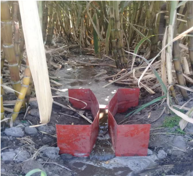
Appendix Figure 7. Field channel and Water measurement by parshall flume
