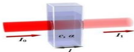
Figure 2.3. The cell containing a solution through which a monochromatic beam of light passes and is partially absorbed by the solution. Where I_0 is the intensity of the incident beam and I_t is the intensity of the transmitted beam.
