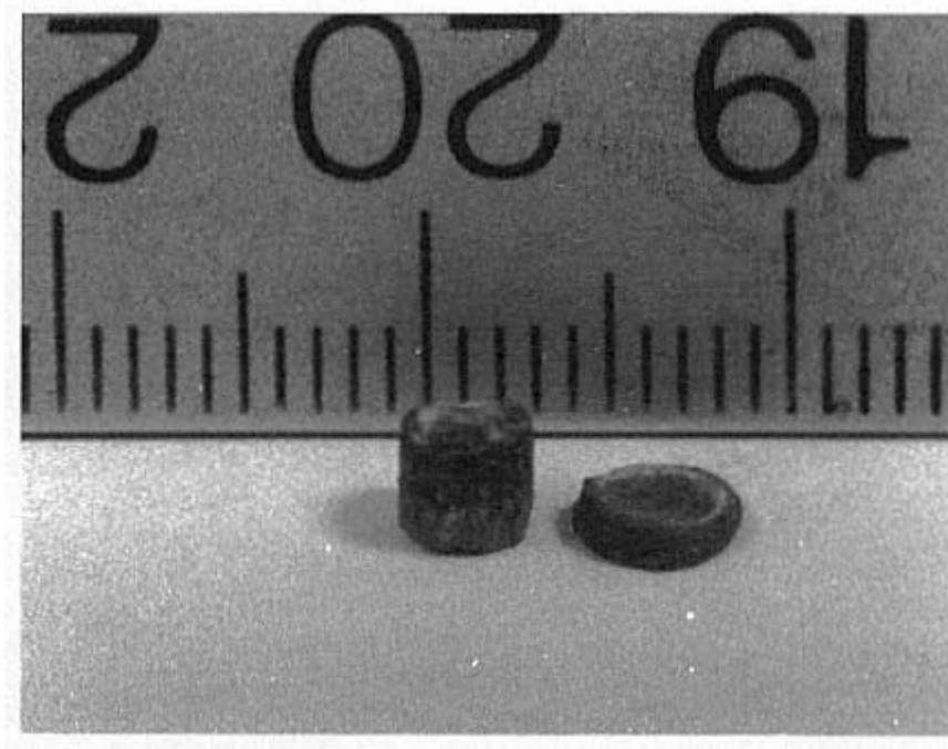
Figure 13.11 Deformation of nanocrystalline \text{TiO}_2 at \approx 800^\circ\text{C} . (From [58].)
