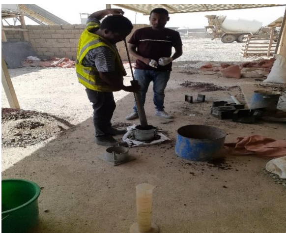
Figure 3.3 C) Modified proctor test
