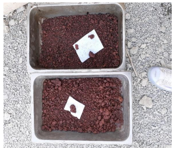
Figure 3.3D) Washed samples of lateritic gravel
