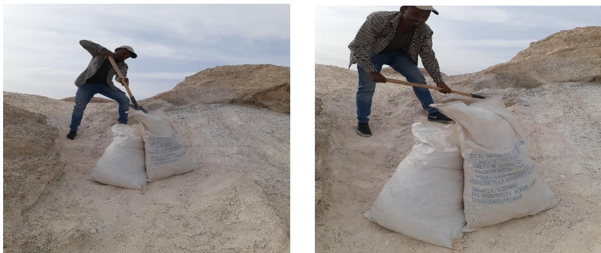
Figure 3. 5 Extracting sample of PCC
