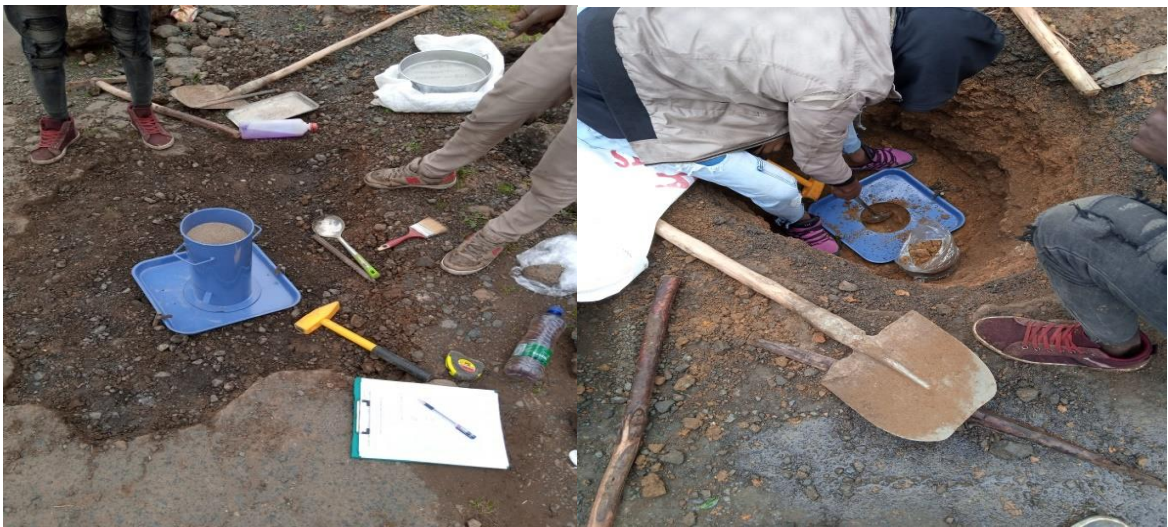
Figure 3-2 Field density determination and thickness measurements.
