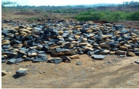
Figure 4.15 Crushed Manually in Mechisho Crushing Site
