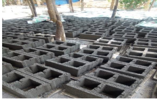
Figure 4.30 - placing of HCB in zemenu HCB production
