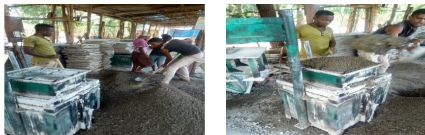
Figure 4.29 - molding of HCB in zemenu HCB production
