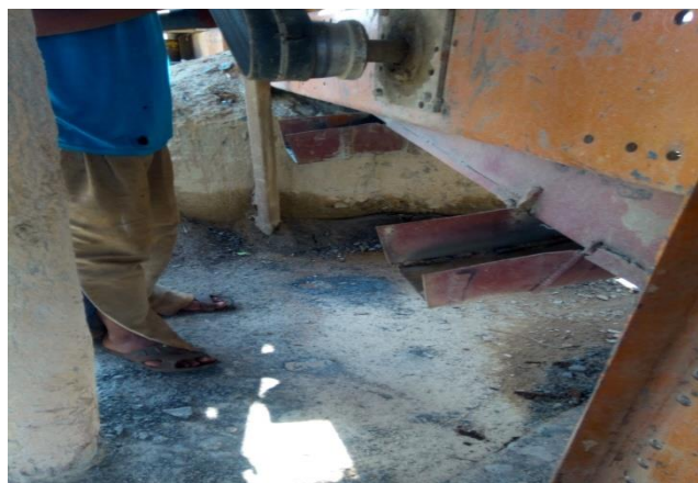
Figure 4.13 the Outlet of Each Size Aggregates
