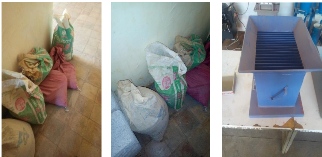
Figure 3.2 Samples and Sample Splitter for Sample Preparation
