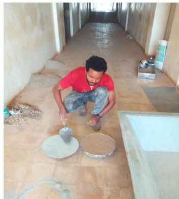
Coping of HCB for Compressive Strength Test
