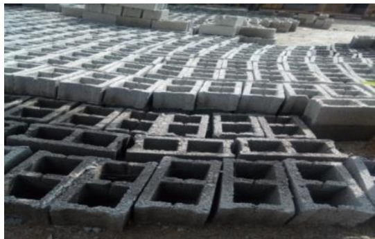
Figure 4.31 - curing of HCB in zemenu HCB production
