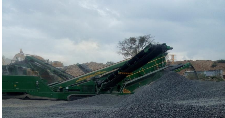
Figure 4.4 the screen (S- 190) on wenago crushing site
