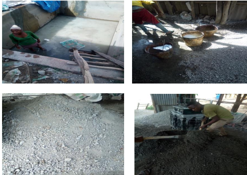
Figure 4.28 - water storage and mixing process in zemenu HCB production
