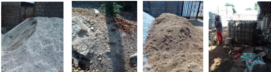
Figure 4.32 - komich, bole, sand and water storage in walelign's hcb production
